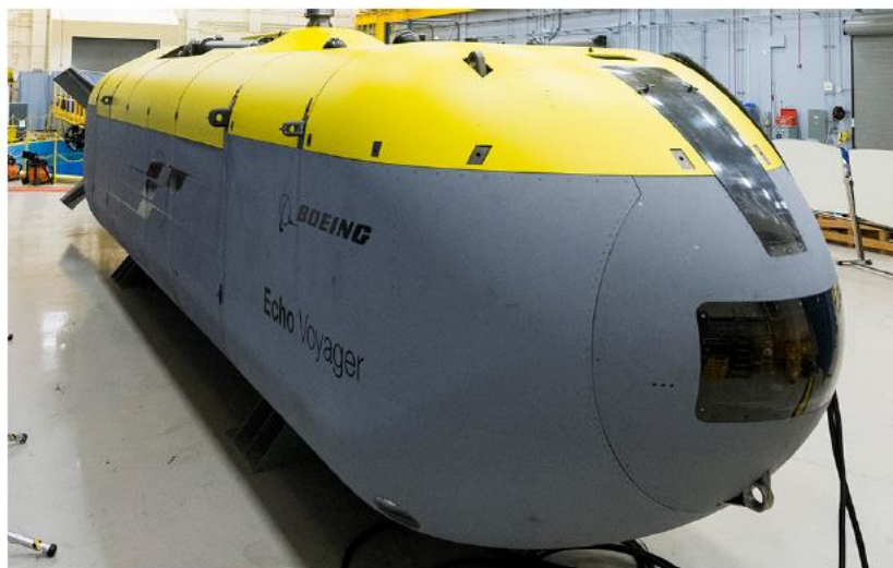
Figure 1: Boeing's Echo Voyager, a precursor to the Orca extra-large UUV. Source: Daniel P. Taylor, CHARTING COURSE ON UUVs. (Sea Power 62, no. 8: October 2019).
