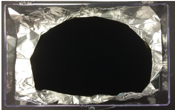
Figure 2: “Vantablack” on equally crinkled tinfoil Open Source: Free Image VantaBlack Image. https://en.wikipedia.org/wiki/Vantablack#/media/File:Vantablack_01.JPG .
