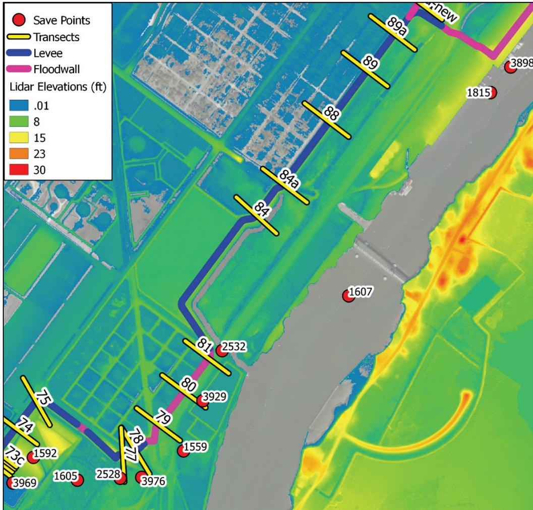
Figure 65. Details of PA-SNWW1, north end, for Port Arthur floodwall (pink), levee (blue), analysis sections (yellow lines), regional modeling output locations (red dots), and color-shaded LiDAR-based elevations (feet, NAVD88).
