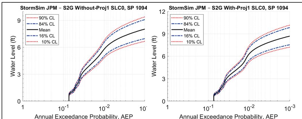
Figure 20. Hazard curves for combined measured SWL and TC minima at SP 1094 for with-project SLC0 scenario.
