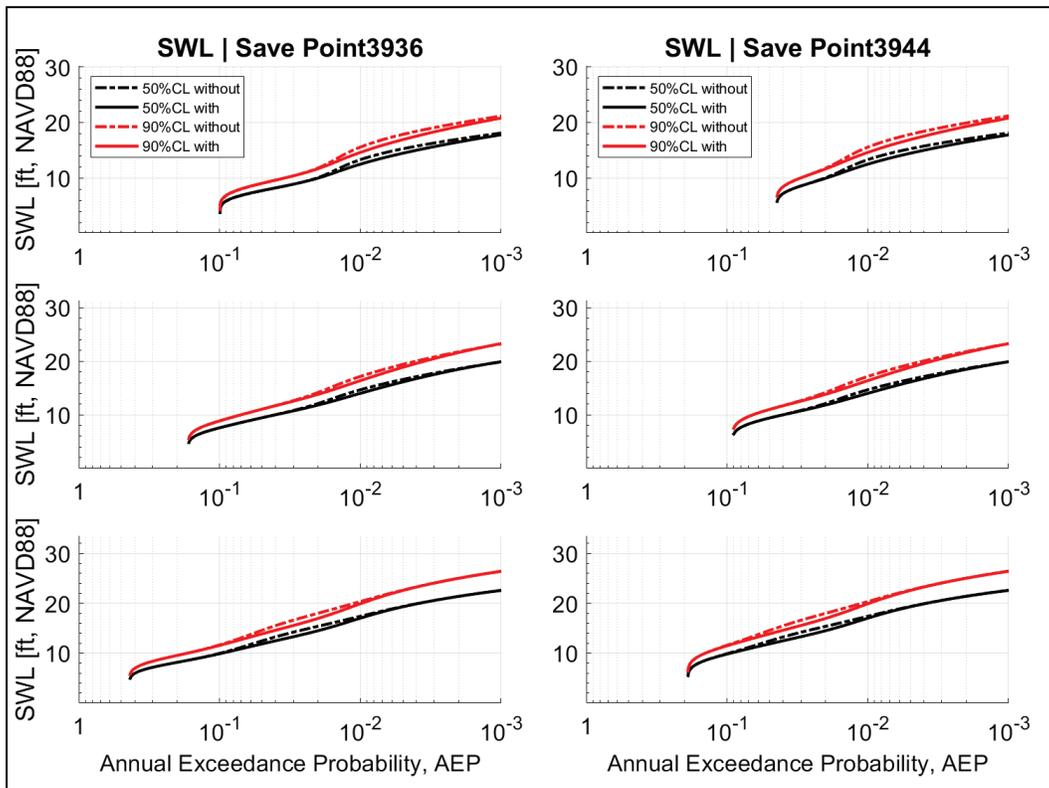
Figure 15. AEP vs.  $H_{m0}$  for SP 3936 (left) and SP 3944 (right). Upper row is SLC0, middle row is SLC1, and bottom row is SLC2.
