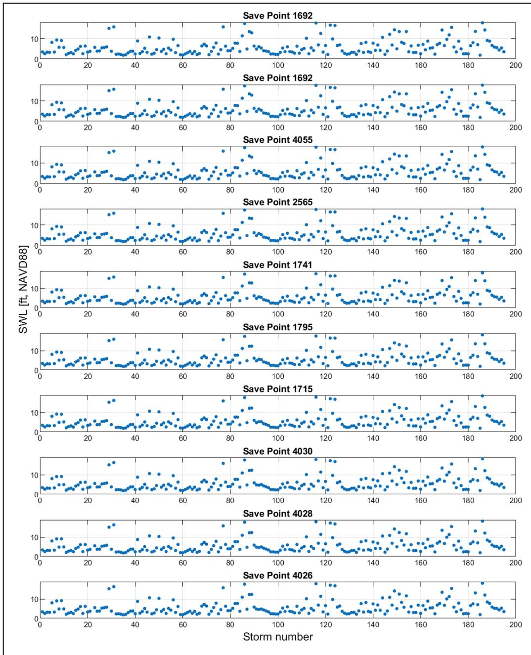
Figure A-19. Peak SWL for with-project and SLC1 for SPs in PA-SNWW2 area. SWL is in feet, NAVD88.
