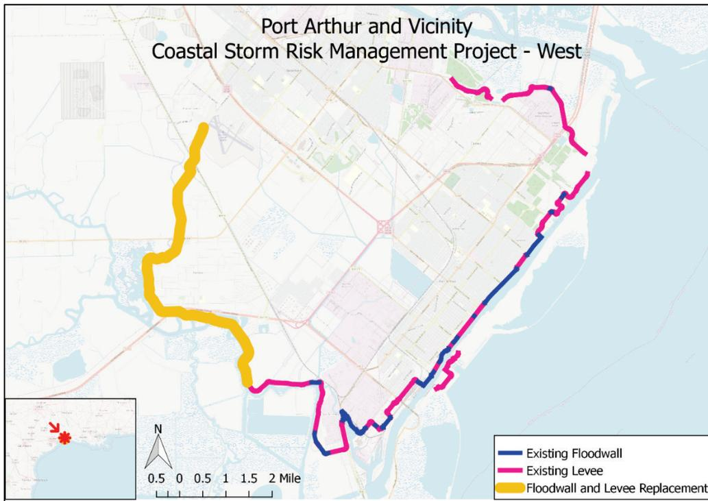
PA-W begins at STA 1139+50 and proceeds to STA 1609+00. Modifications include increasing levee, pump station fronting protection, and gate crest elevations.
