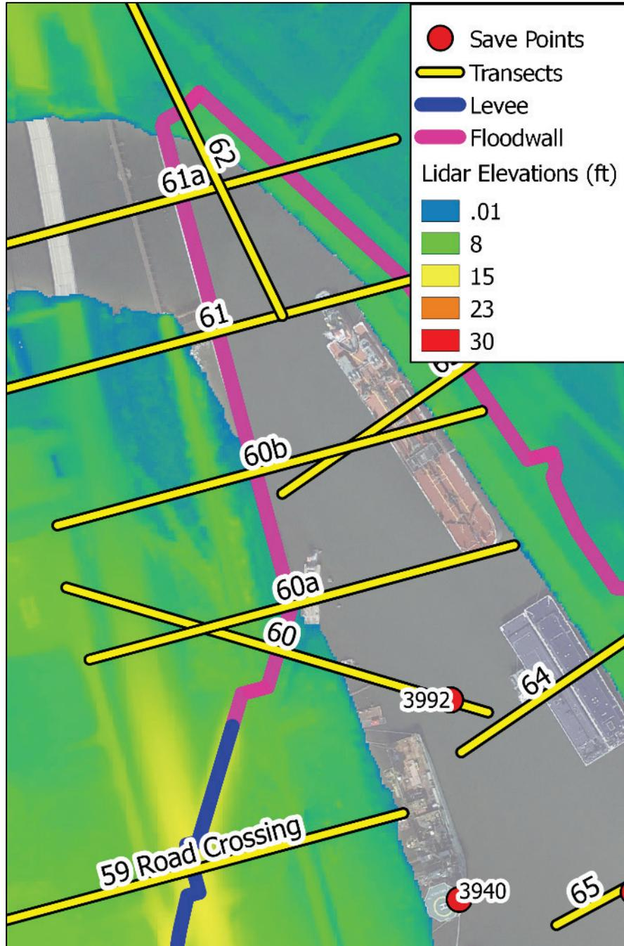
A 76 m portion of the floodwall shown in Figure 28 was damaged prior to hurricane Harvey in August 2017. The damage was attributed to scour on the floodside at the toe of the wall caused by propeller wash from berthing maneuvers of ships in the turning basin.
