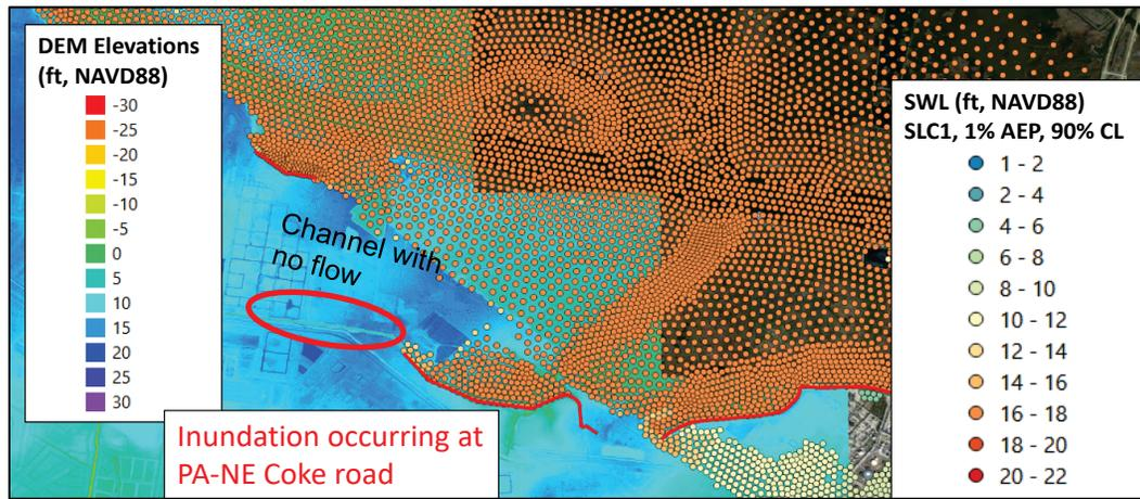
Figure 109. Inundation shown behind levee at the north end of PA-NE, color-shaded LiDAR-based elevations (feet, NAVD88), and colored regional nodal output locations corresponding to the SWL for SLC2 at 1% AEP, 50% CL.
