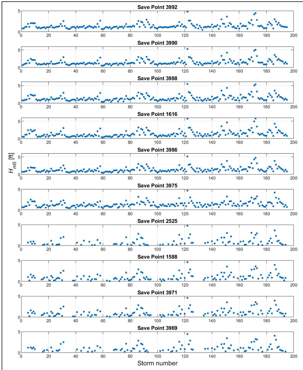
Figure B-7. Peak  $H_{m0}$ , in feet, for with-project and SLC2 for SPs in Contract 3 area.
