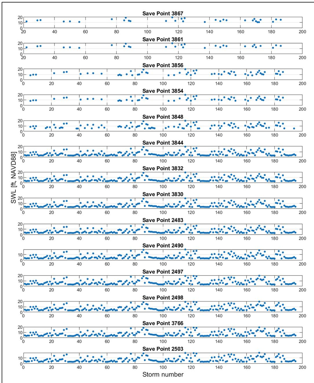
Figure A-11. Peak SWL for with-project and SLC2 for SPs in PA-W area. SWL is in feet, NAVD88.
