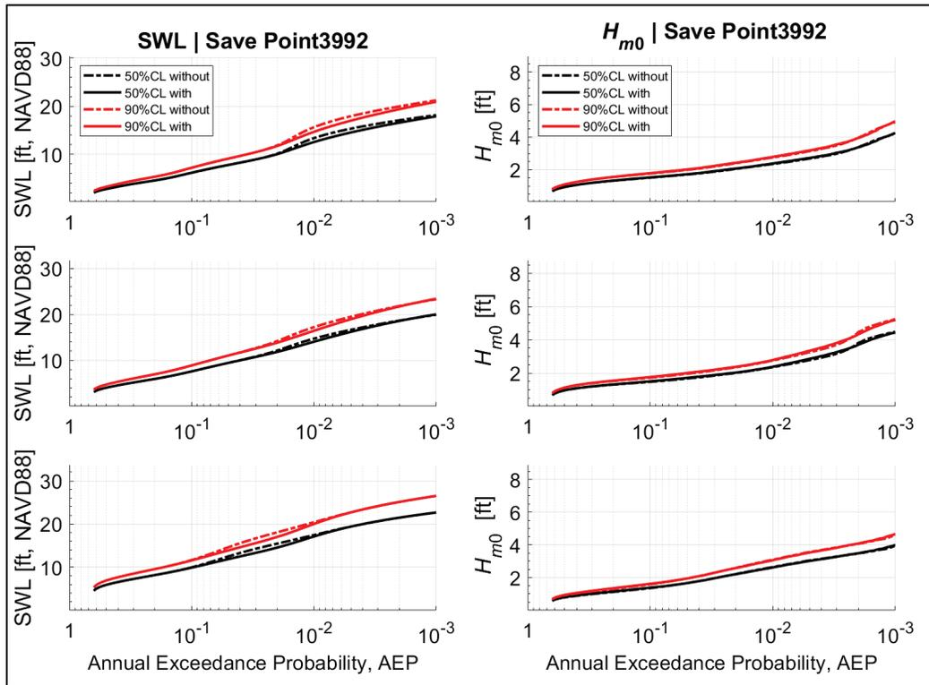
Comparing the hazards for SWL and  $H_{m0}$ , it can be seen that while there are differences between with-project and without-project individual storm responses, these differences have almost no effect on the hazards. There is some difference in SWL near 1% AEP. These differences may be attributed to the change in flood patterns with the modifications of CSRM structures and local navigation channels.
