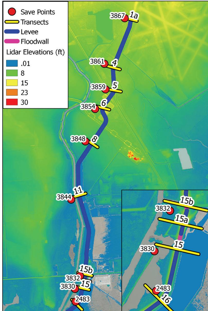
Figure 47. Details of PA-W, south end, for Port Arthur floodwall (pink), levee (blue), analysis sections (yellow lines), regional modeling output locations (red dots), and color-shaded LiDAR-based elevations (feet, NAVD88).
