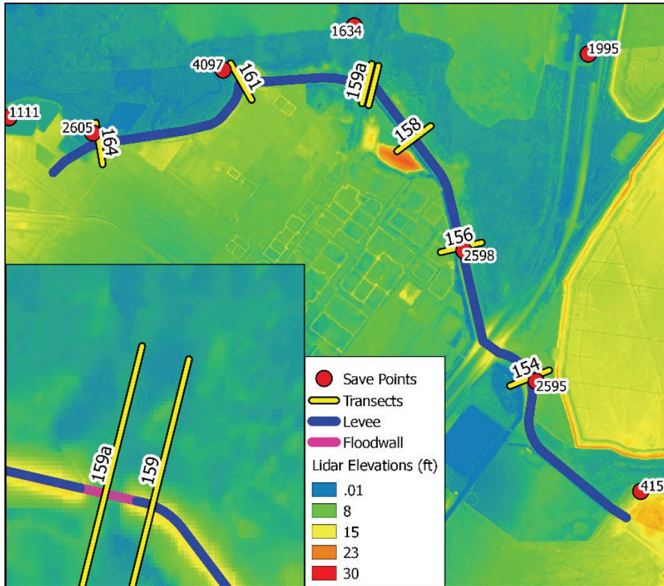
Figure 92. Details of PA-NE, west end, for Port Arthur levee (blue), analysis sections (yellow lines), regional modeling output locations (red dots), and color-shaded LiDAR-based elevations (feet, NAVD88).
