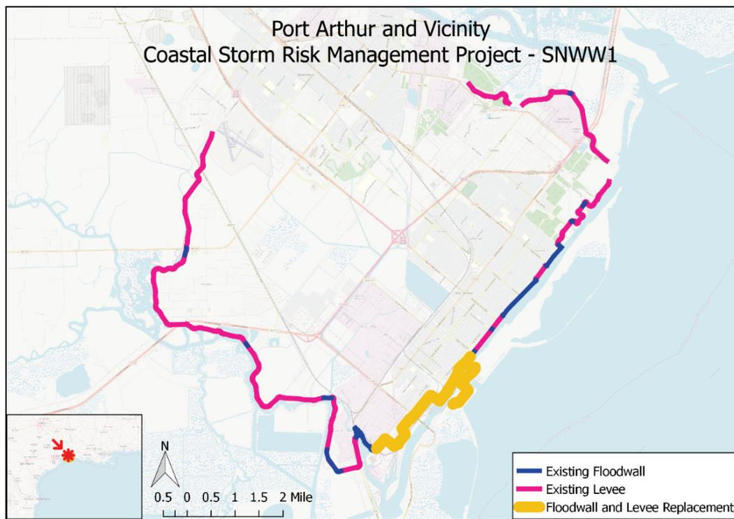
The south half of PA-SNWW1 begins at STA 653+00.00 and proceeds to STA 762+13.00. The northern half of PA-SNWW1 begins at STA 569+60.00 and proceeds to STA 617+53.11. Structure modifications include increasing the elevations of both the floodwall and levee.
