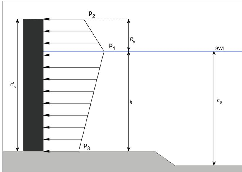
Figure 6. Floodwall fluid hydrodynamic pressure characteristics when SWL is higher than the structure crest elevation (freeboard,  $R_c$ , is negative).
