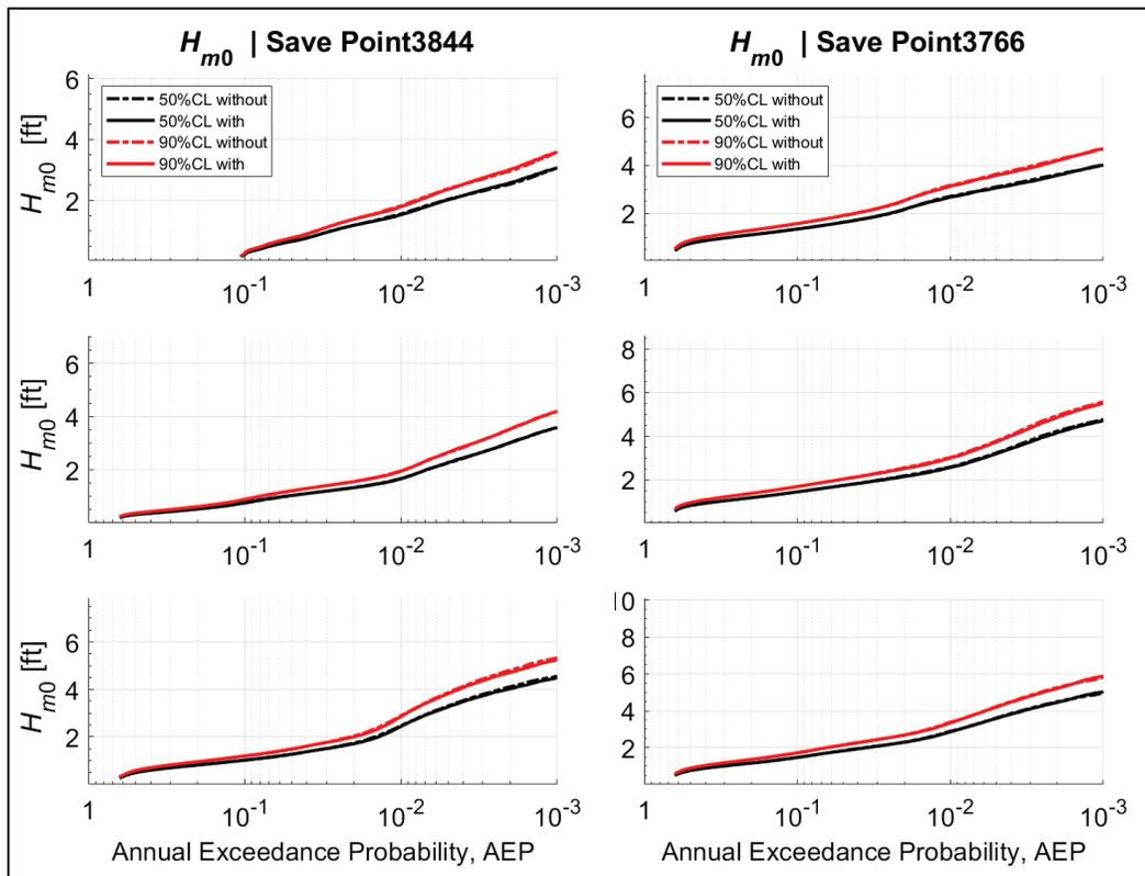
Comparing the hazard curves for SWL and  $H_{m0}$ , it can be seen that while there are differences between with-project and without-project individual storm responses, these differences have almost no effect on the hazards. These differences may be attributed to the change in flood patterns with the modifications of CSRM structures and local navigation channels.
