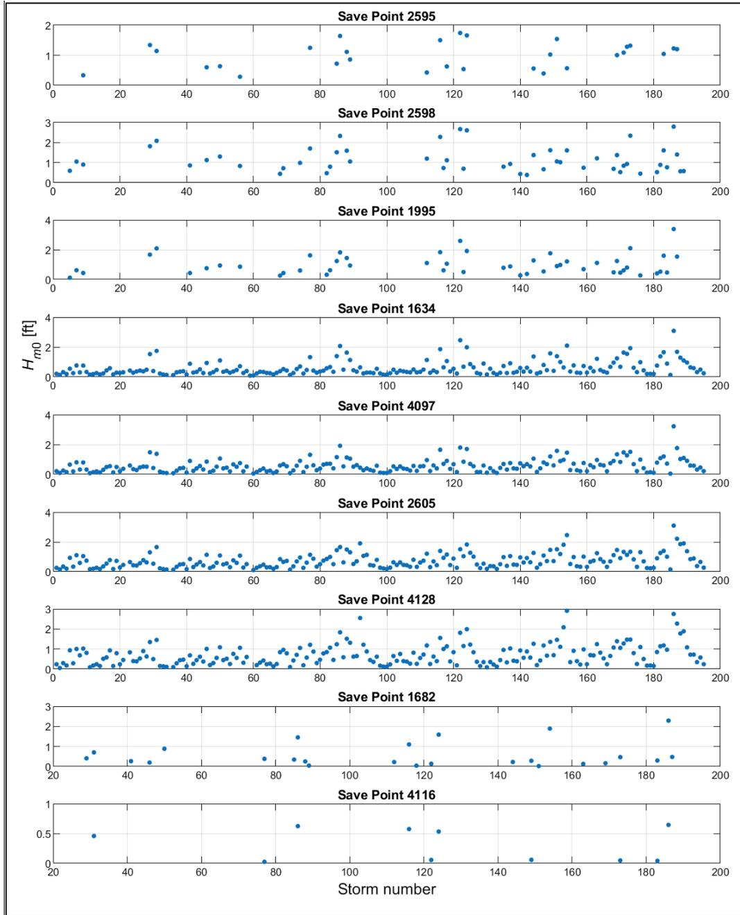
Figure B-25. Peak  $H_{m0}$ , in feet, for with-project and SLC1 for SPs in PA-NE area.
