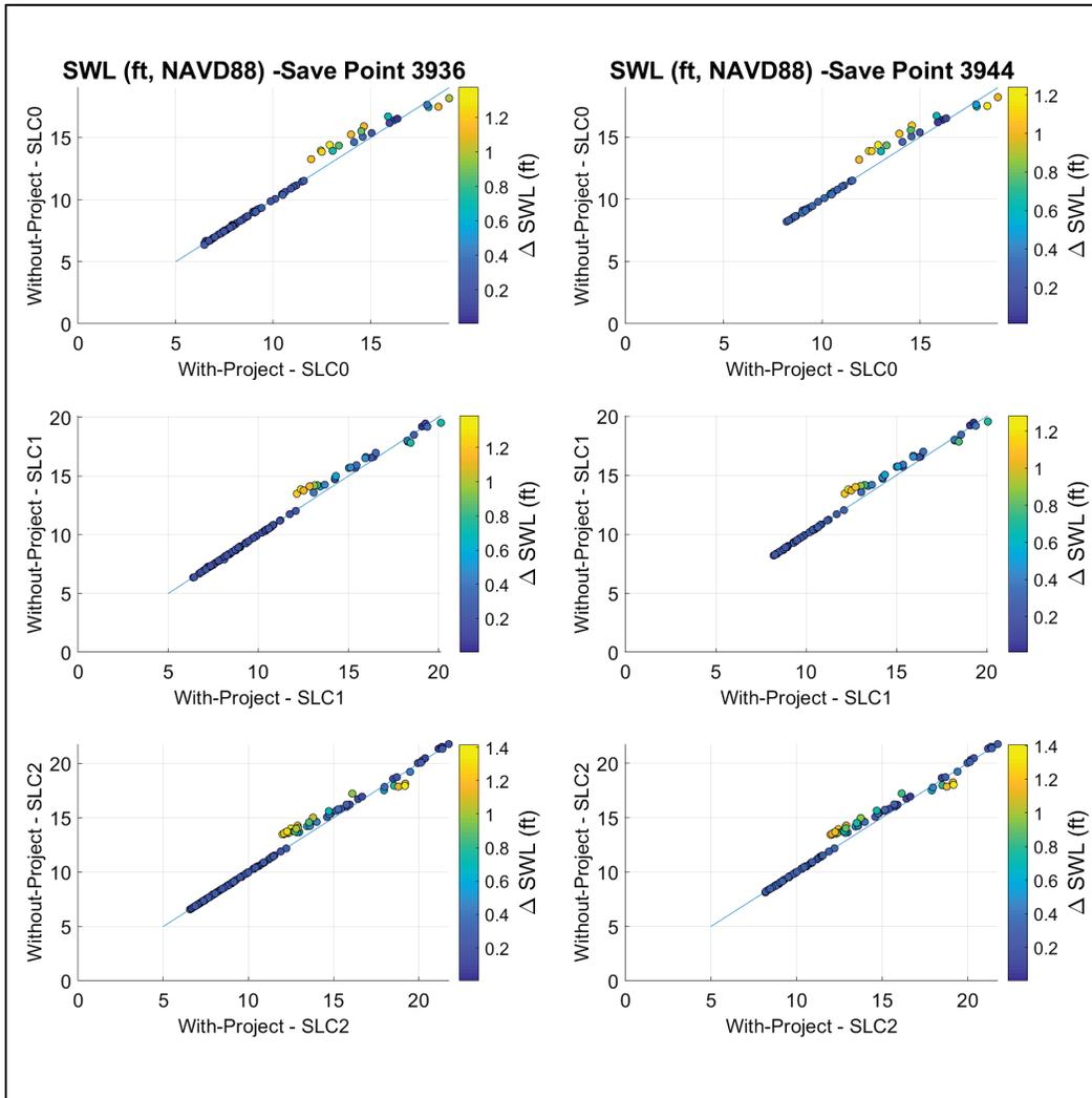
Figure 13. With-project  $H_{m0}$  peaks for all storms plotted against without-project conditions for SPs 3936 (left) and 3944 (right). Upper row is SLC0, middle row is SLC1, and bottom row is SLC2.
