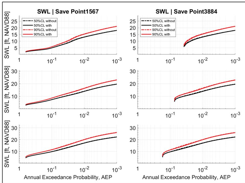
Figure 60. AEP vs.  $H_{m0}$  for SP 1567 (left) and SP 3884 (right). Upper row is SLC0, middle row is SLC1, and bottom row is SLC2.
