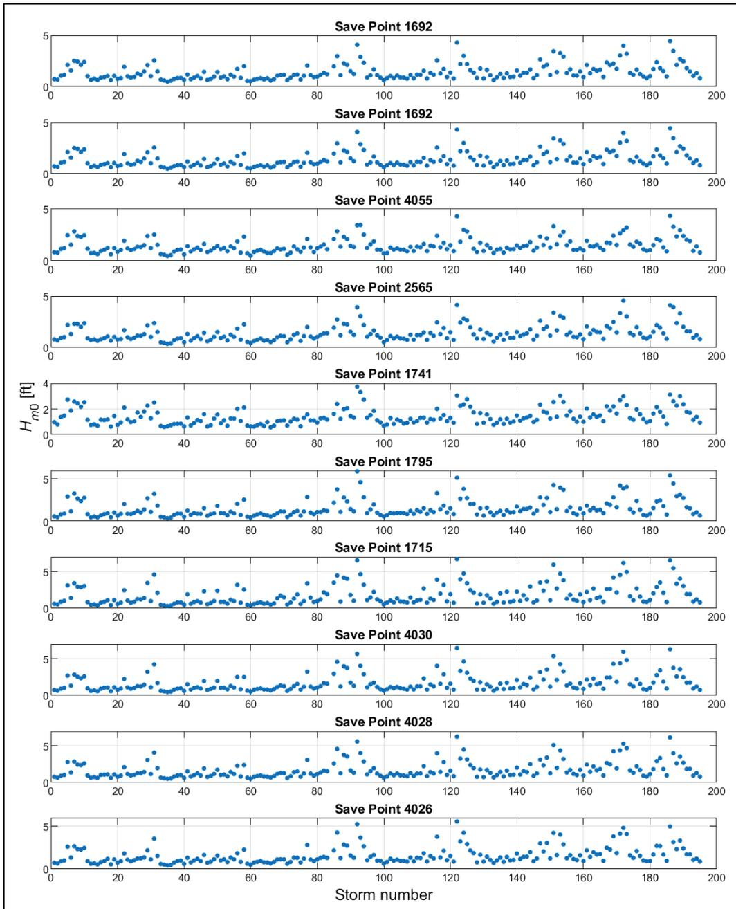
Figure B-20. Peak  $H_{m0}$ , in feet, for with-project and SLC2 for SPs in PA-SNWW2 area.
