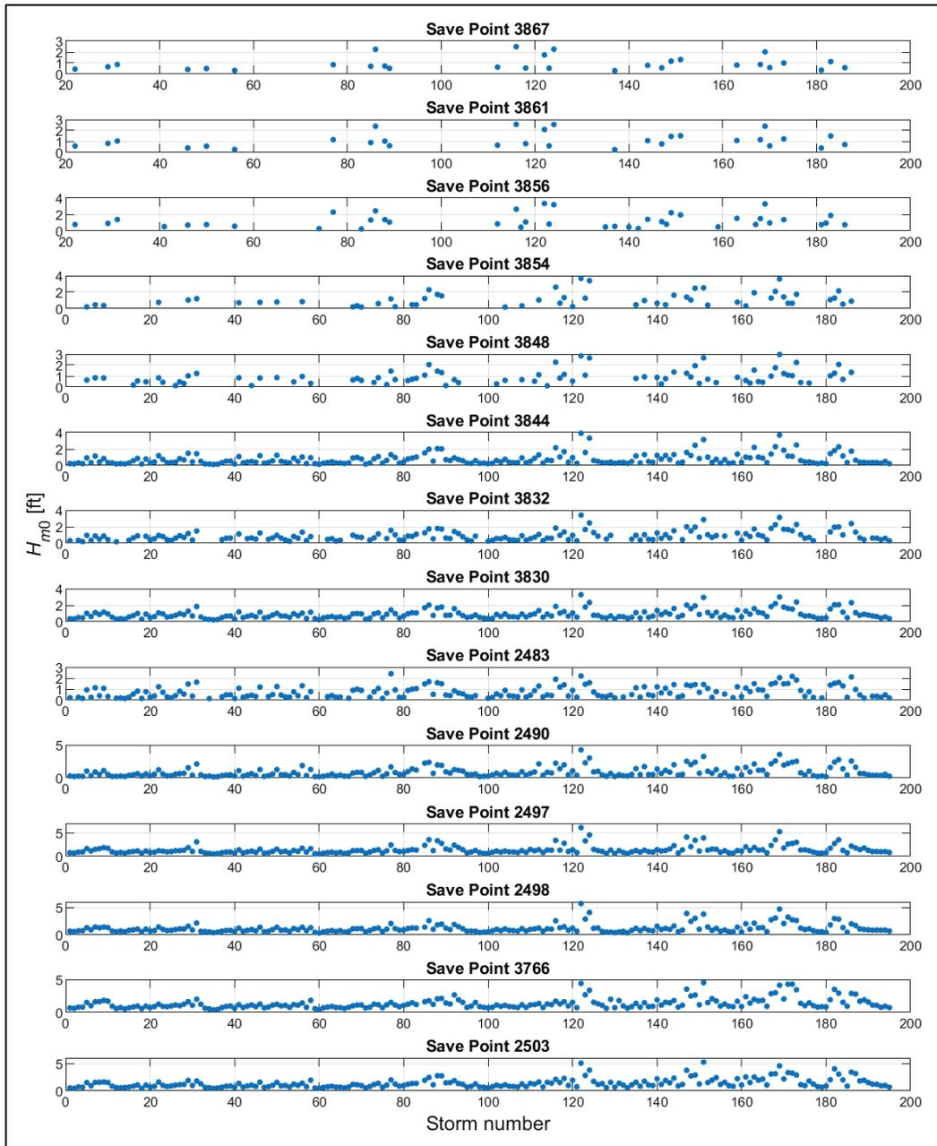
Figure B-11. Peak  $H_{m0}$ , in feet, for with-project and SLC2 for SPs in PA-W area.
