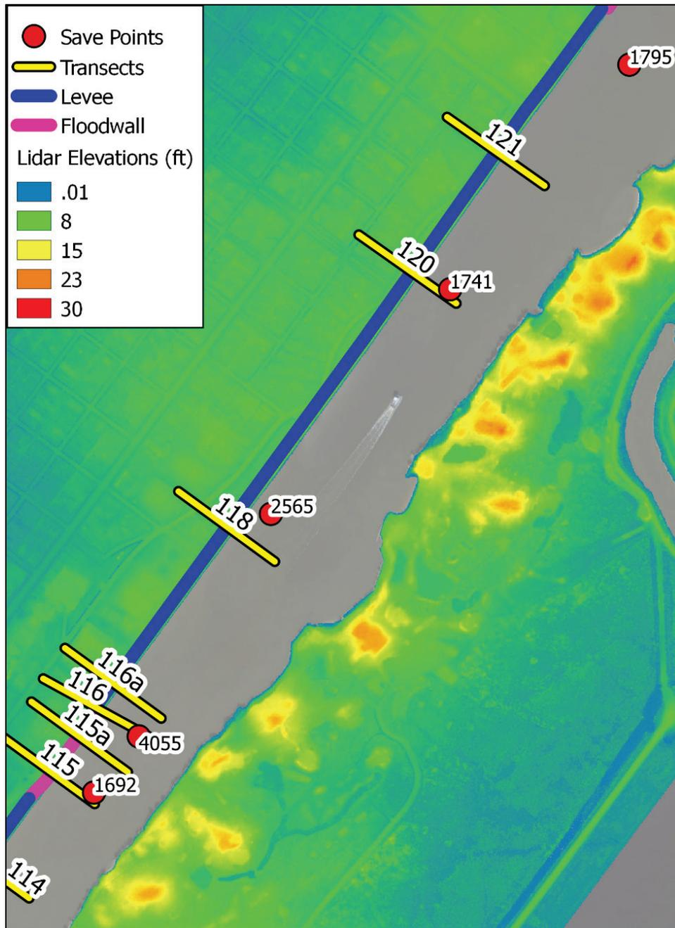
Figure 75. Details of PA-SNWW2, north end, for Port Arthur floodwall (pink), levee (blue), analysis sections (yellow lines), regional modeling output locations (red dots), and color-shaded LiDAR-based elevations (feet, NAVD88).
