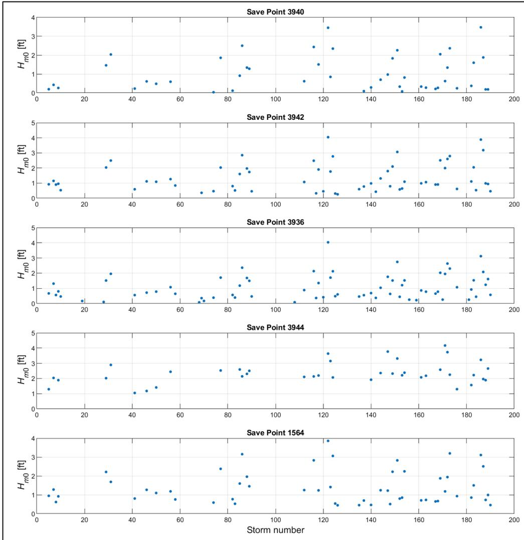
Figure B-2. Peak  $H_{m0}$ , in feet, for with-project and SLC1 for SPs in Contract 1 area.
