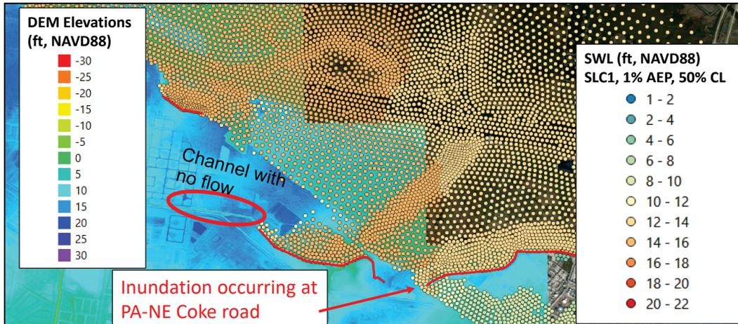
Figure 108. Inundation shown behind levee at PA-NE Coke Road, color-shaded LiDAR-based elevations (feet, NAVD88), and colored regional nodal output locations corresponding to the SWL for SLC1 at 1% AEP, 90% CL.
