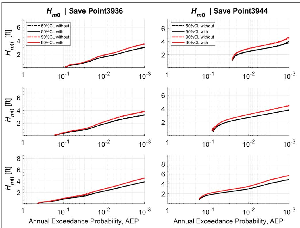
Comparing the hazards for SWL and  $H_{m0}$ , it can be seen that while there are some differences between with-project and without-project individual storm responses, these differences have almost no effect on the hazards. These differences for individual storm responses may be attributed to the change in flood patterns with the modifications of CSRM structures and local navigation channels.
