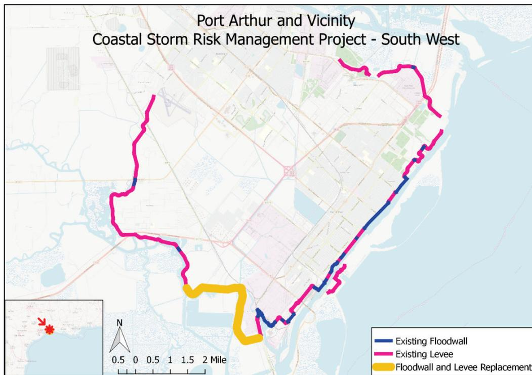
The PA-SW portion of Port Arthur includes a section of the existing CSRSM system of floodwall pump station fronting protection and levee along the Port of Port Arthur, shown in Figure 56. The contract begins at STA 933+80.00 and proceeds to STA 1139+50.00.
