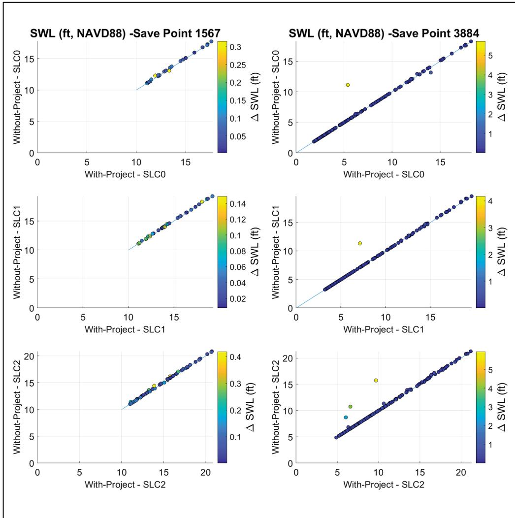
Figure 58. With-project  $H_{m0}$  peaks for all storms plotted against without-project conditions for SPs 1567 (left) and 3884 (right). Upper row is SLC0, middle row is SLC1, and bottom row is SLC2.
