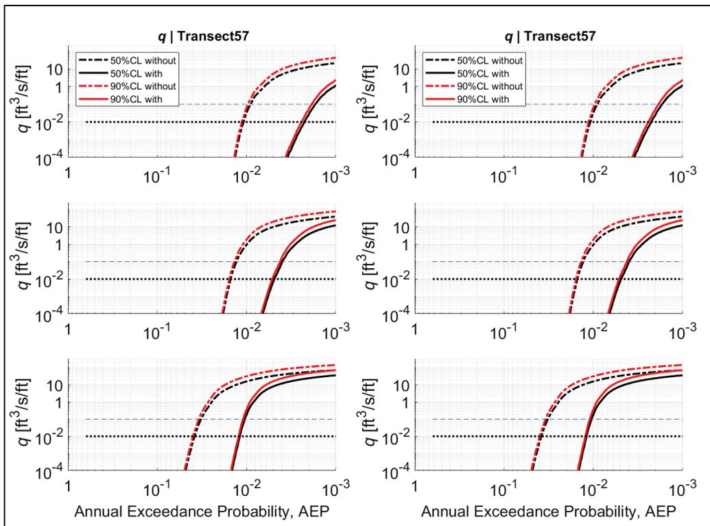
The overtopping distributions above are generally steep over the higher frequency half and intersect the lower horizontal axis slightly less than the 1% AEP for with-project, suggesting that there is no overtopping for high
