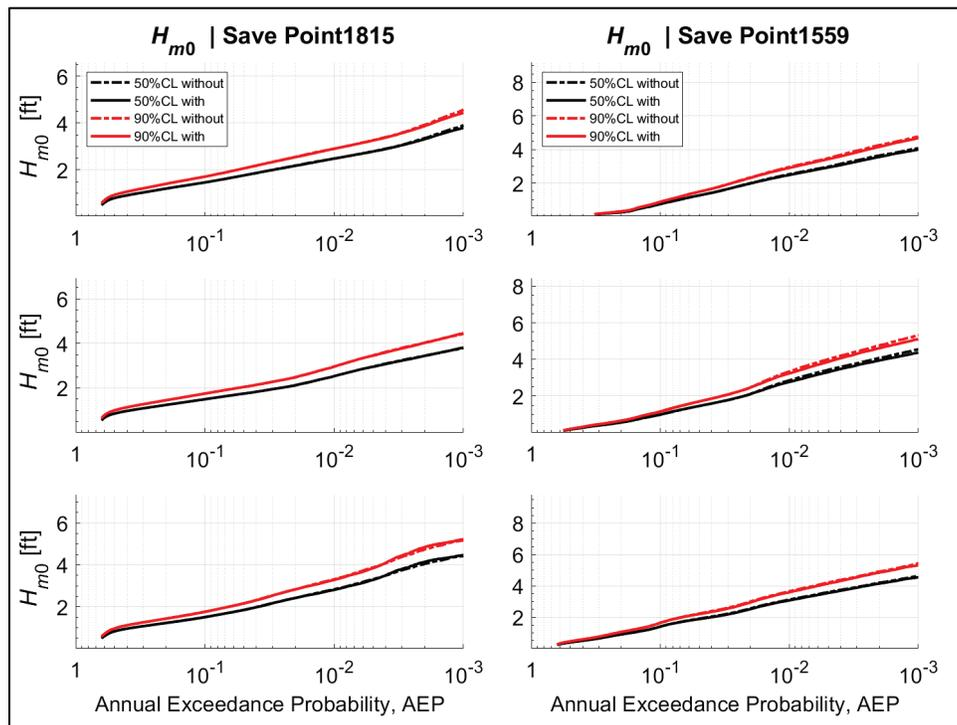
Comparing the hazard curves for SWL and  $H_{mo}$ , it can be seen that while there are differences between with-project and without-project individual storm responses, these differences have almost no effect on the hazards. These differences may be attributed to the change in flood patterns with the modifications of CSRM structures and local navigation channels.
