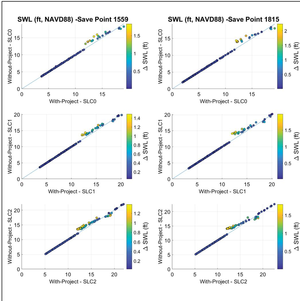
Figure 67. With-project  $H_{m0}$  peaks for all storms plotted against without-project conditions for SPs 1559 (left) and 1815 (right). Upper row is SLC0, middle row is SLC1, and bottom row is SLC2.
