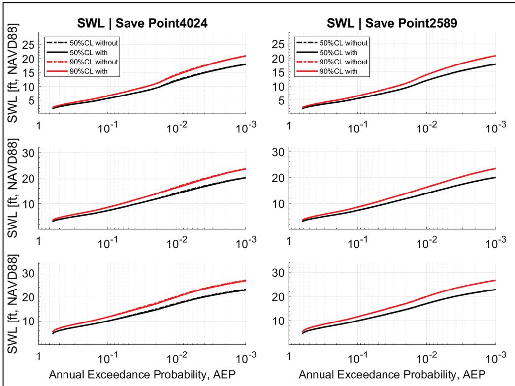
Comparing the hazard curves for SWL and  $H_{mo}$ , it can be seen that while there are differences between with-project and without-project individual storm responses, these differences have almost no effect on the hazards.
