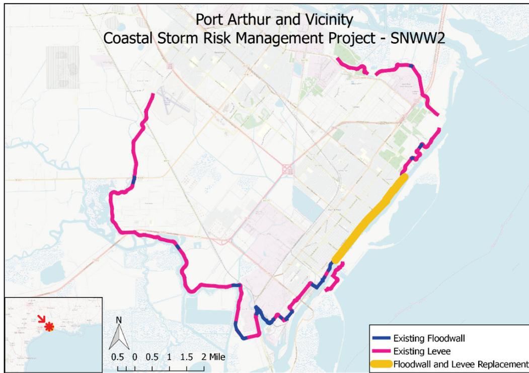
The PA-SNWW2 area for Port Arthur includes a section of the existing CSRM system along the SNWW, shown Figure 74 and Figure 75. The contract begins at STA 385+12.00 and proceeds to STA 561+60.00. Structure modifications include increasing the elevations of both the floodwall and levee.
