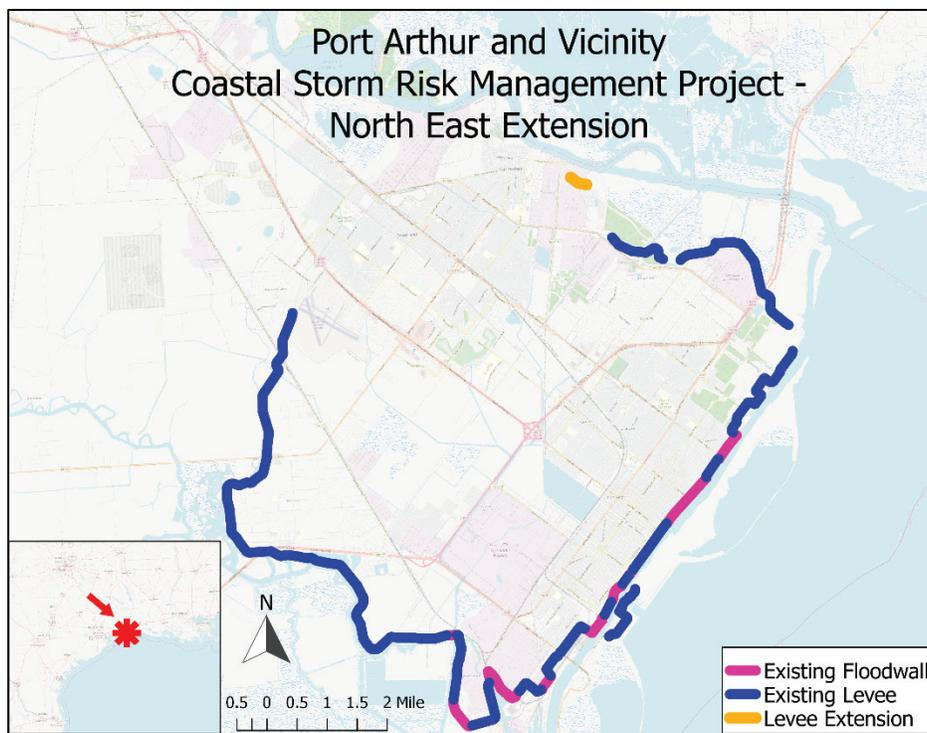
Figure 100. Details of PA-NE-ext for Port Arthur levee (blue), analysis sections (yellow lines), regional modeling output locations (red dots), and color shaded LiDAR-based elevations (feet, NAVD88).
