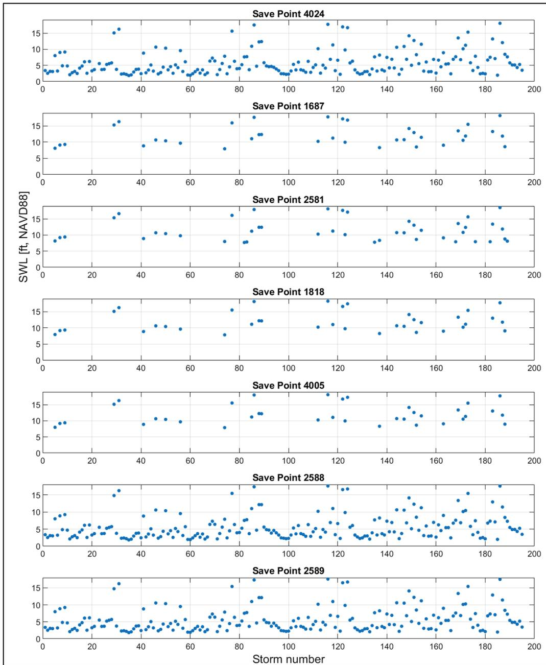
Figure A-22. Peak SWL for with-project and SLC1 for SPs in PA-SNWW3 area. SWL is in feet, NAVD88.
