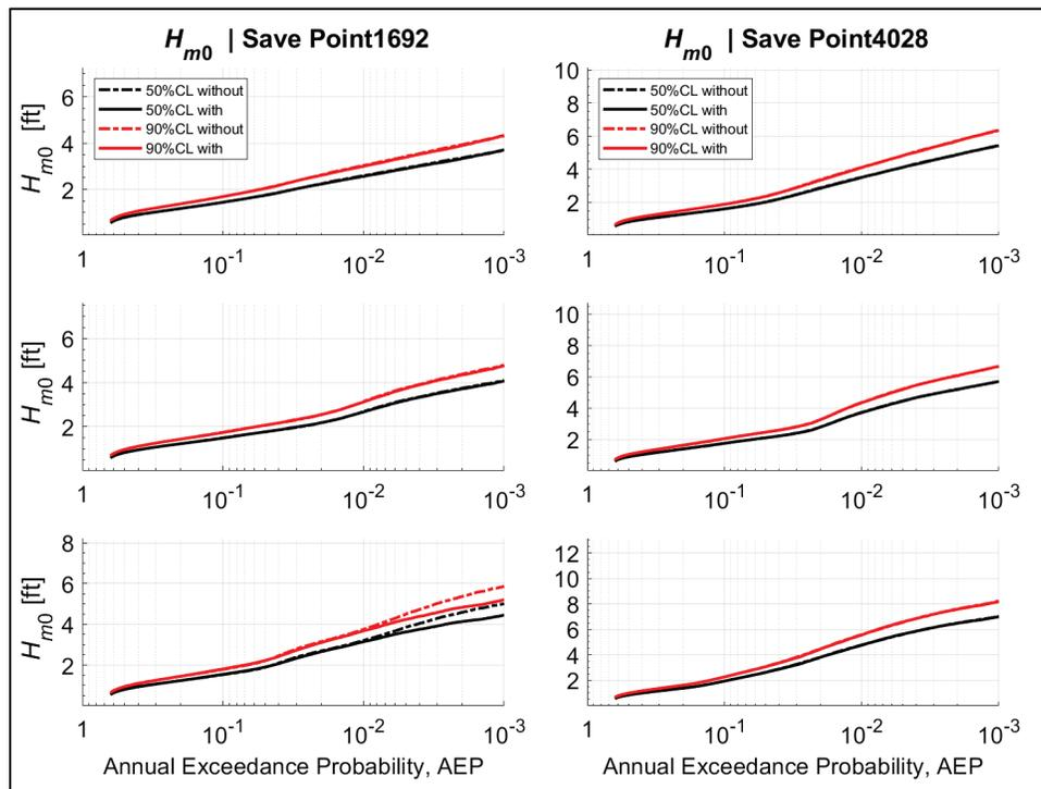
Comparing the hazard curves for SWL and  $H_{mo}$ , it can be seen that while there are differences between with-project and without-project individual storm responses, these differences have almost no effect on the hazards. These differences may be attributed to the change in flood patterns with the modifications of CSRMs structures and local navigation channels.
