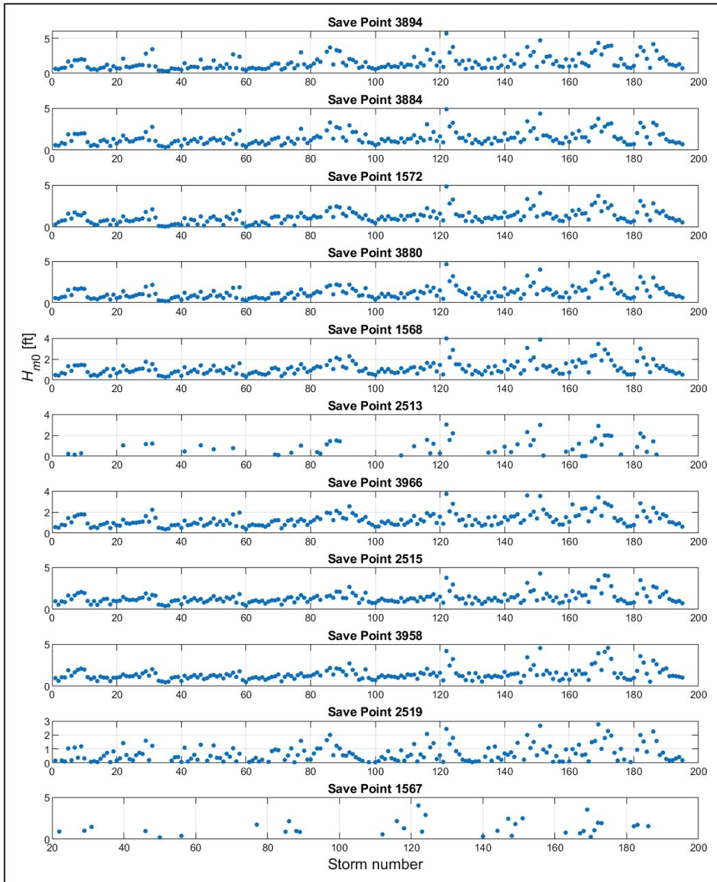
Figure B-14. Peak  $H_{m0}$ , in feet, for with-project and SLC2 for SPs in PA-SW area.
