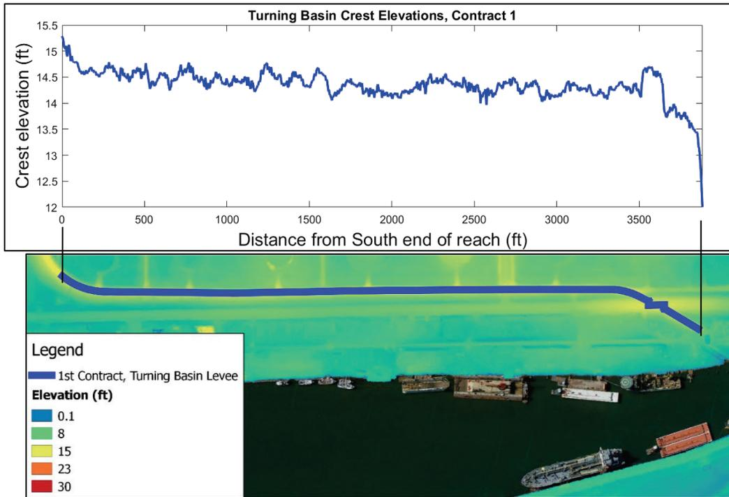
Figure 22. West reach without-project levee crest elevations relative to NAVD88.
