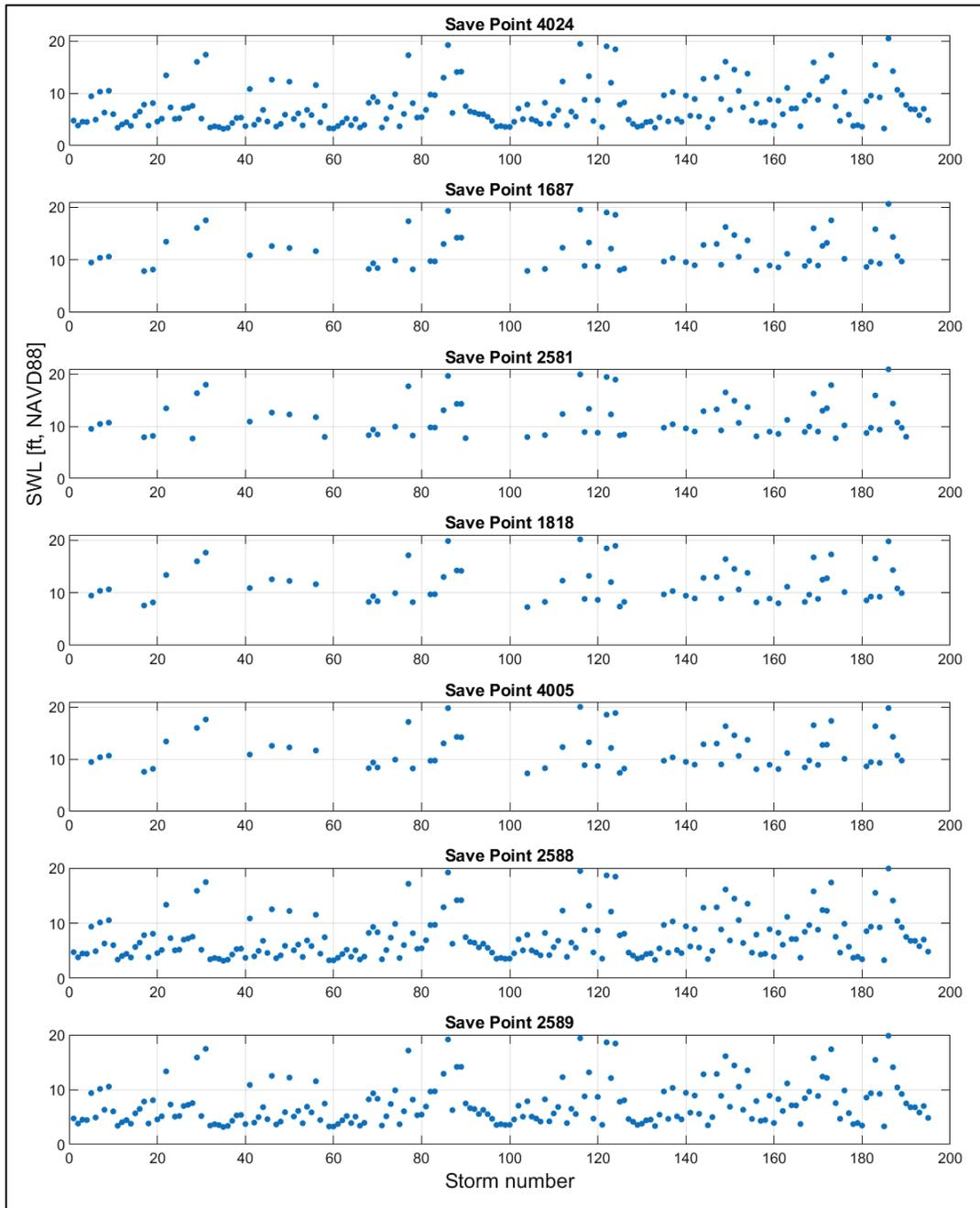
Figure A-23. Peak SWL for with-project and SLC2 for SPs in PA-SNWW3 area. SWL is in feet, NAVD88.
