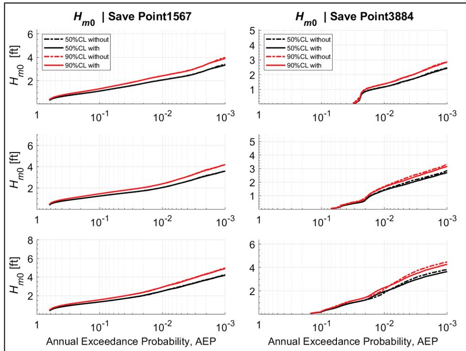
Comparing the hazard curves for SWL and  $H_{mo}$ , it can be seen that while there are differences between with-project and without-project individual storm responses, these differences have almost no effect on the hazards. These differences may be attributed to the change in flood patterns with the modifications of CSRSM structures and local navigation channels.
