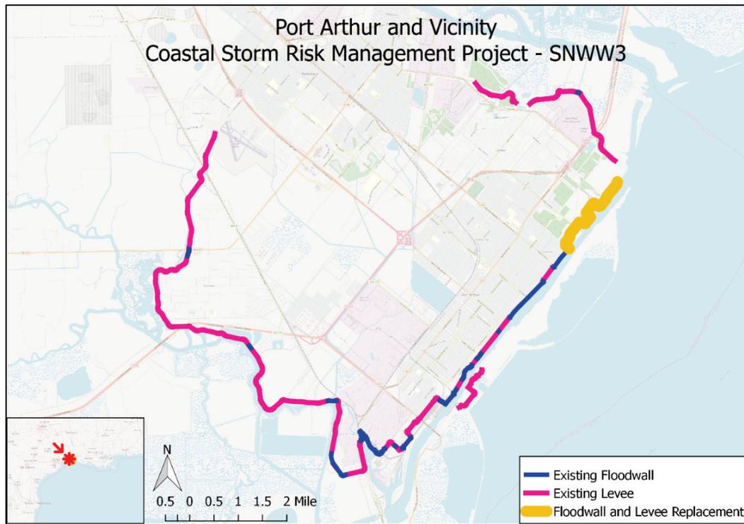
The PA-SNWW3 area for Port Arthur includes a section of the existing CSRM system along the SNWW, shown in Figure 83. The contract begins at STA 258+15.00+00 and proceeds to STA 381+30.00. Structure modifications include increasing the elevations of both the floodwall and levee.
