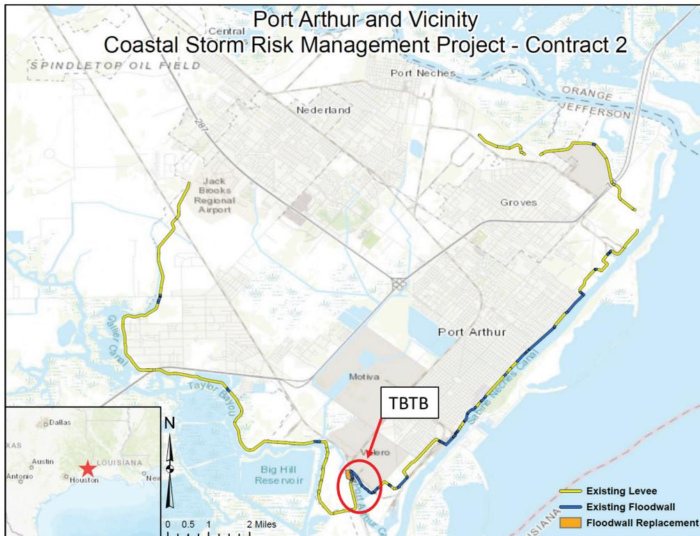
Figure 27. Details of Contract 2 for Port Arthur floodwall (pink), levee (blue), analysis sections (yellow lines), regional modeling output locations (red dots), and color-shaded LiDAR-based elevations (feet, NAVD88).
