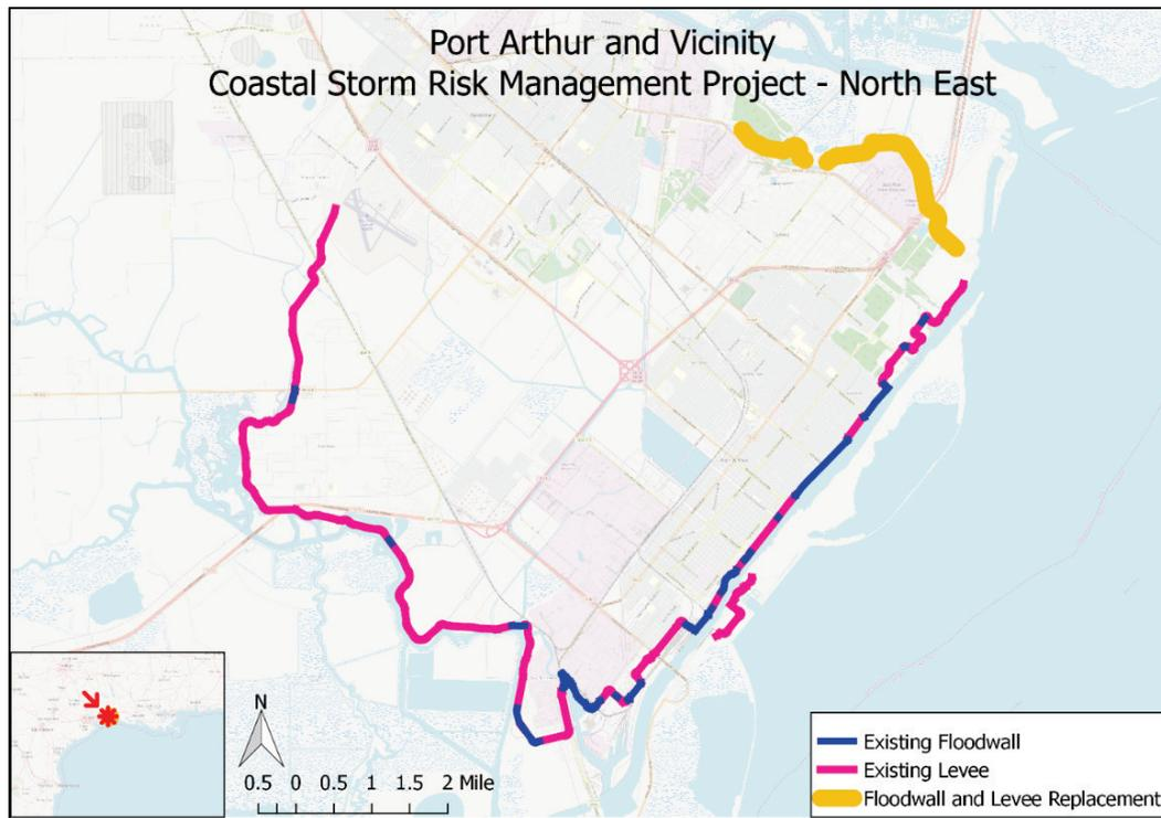
The PA-NE area for Port Arthur includes a section of the existing CSRM system along the northeast edge of Port Arthur, shown Figure 91 and Figure 92. The contract begins at STA 00+00 and proceeds southeast to STA 230+55. The contract includes increasing structure crest elevations.
