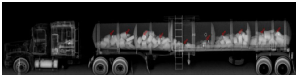
X-Ray Image of a Commercial Vehicle with Indicators of Contraband Smuggling
