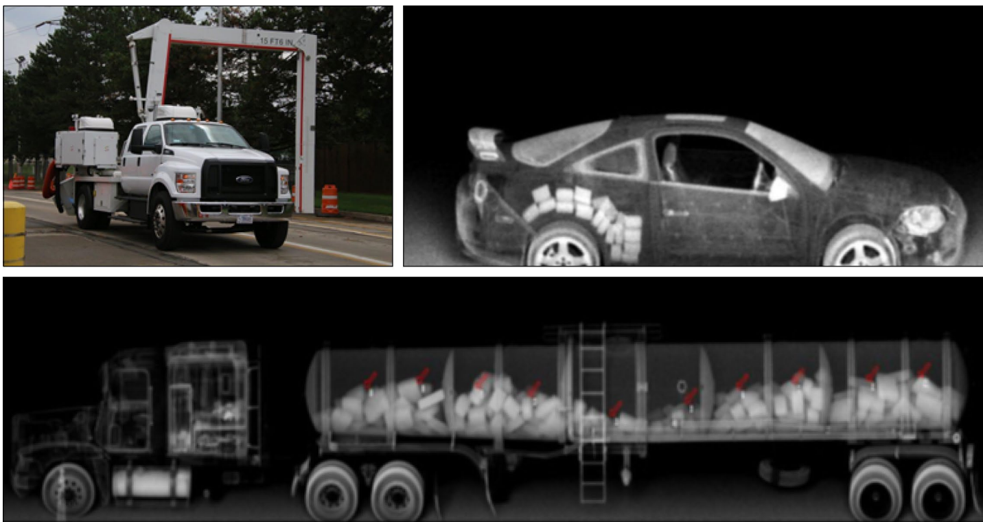
Figure 7: Non-Intrusive Inspection Equipment and Vehicle Scans Showing Indicators of Contraband Smuggling
