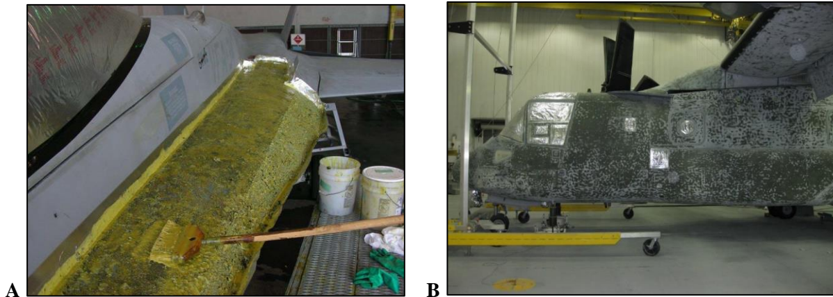
Figure 1 — Removal of polyurethane topcoats on Navy aircraft using a) a methylene chloride based chemical stripper and b) hand-sanding with abrasive paper.
