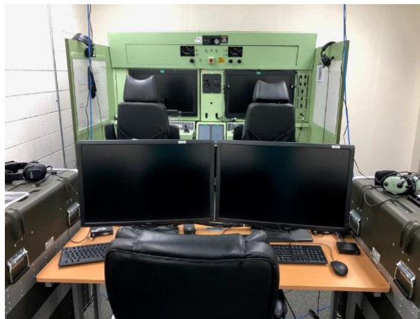
Figure 1. Army's Universal Mission Simulator with the operator's console in the foreground.
