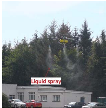
Figure 1: Crop spray drone hovering. The liquid spray is seen below the drone.
