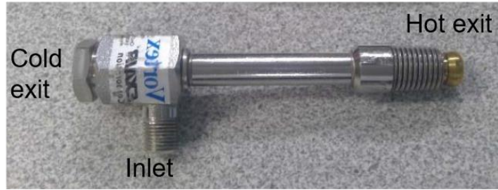
Figure 45. Commercial vortex tube, Exair™ 3208
