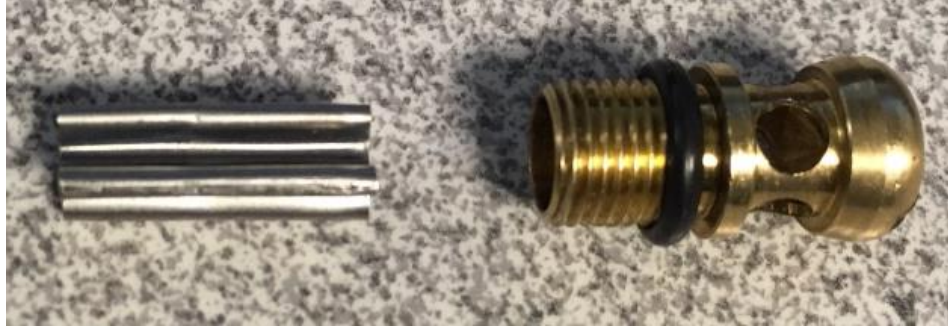
Figure 83. Exair™ 3208 vortex tube cruciform insert (left) and original hot exit geometry (right)
