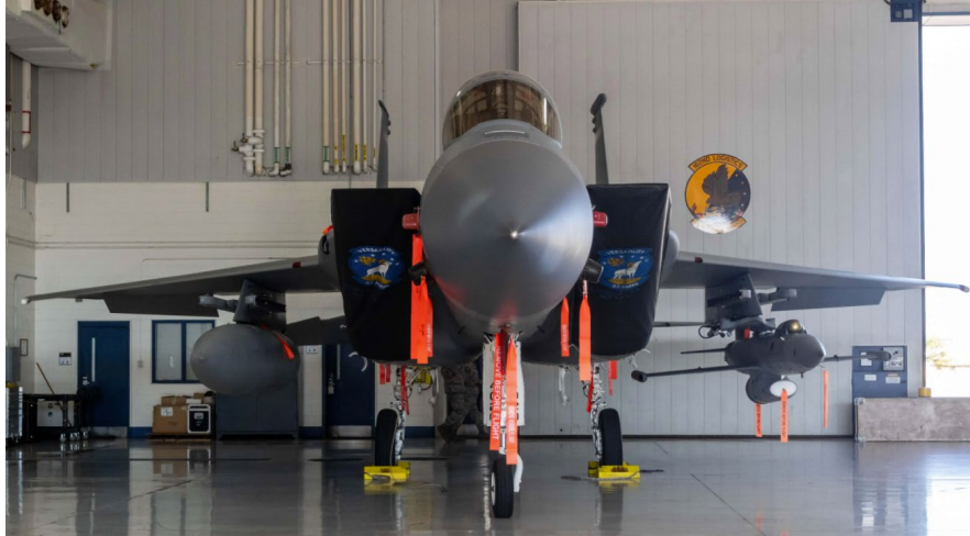
Figure 8. F-15C with UTAP-22 Drone attached to the left pylon (Newdick, 2021)
