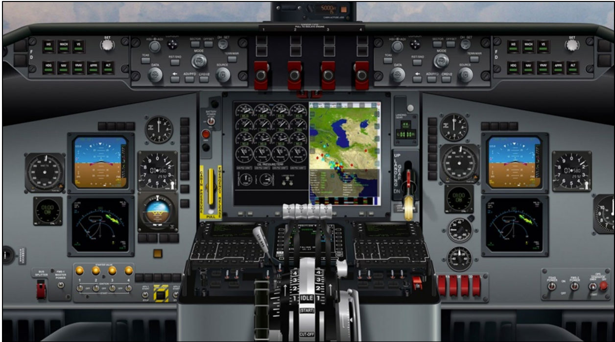
Figure 5. KC-135R RTIC Block 45 Electronic Engine Instrument Display (EEID) and moving map ( Rockwell Collins to Implement RTIC System for USAF's KC-135R Tankers, 2018 )
