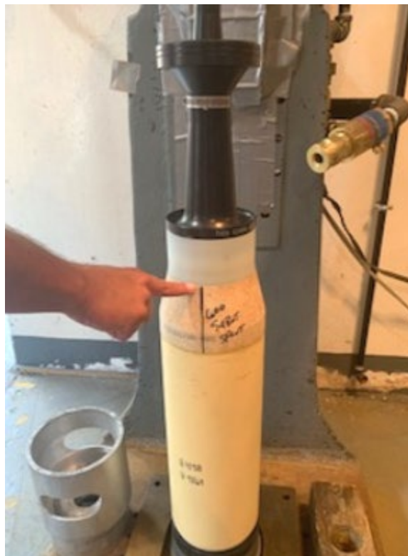
Fig. 11 Complete assembly of the projectile into the case adapter
