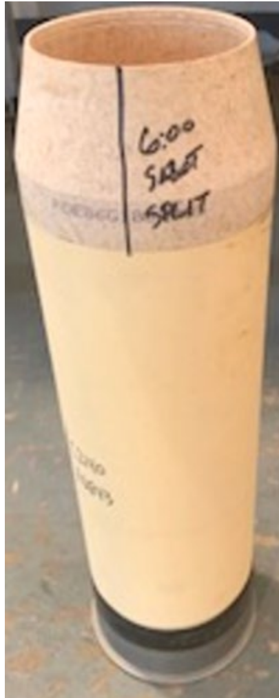
Fig. 6 6 o'clock sabot split alignment markings on combustible case and case adapter
