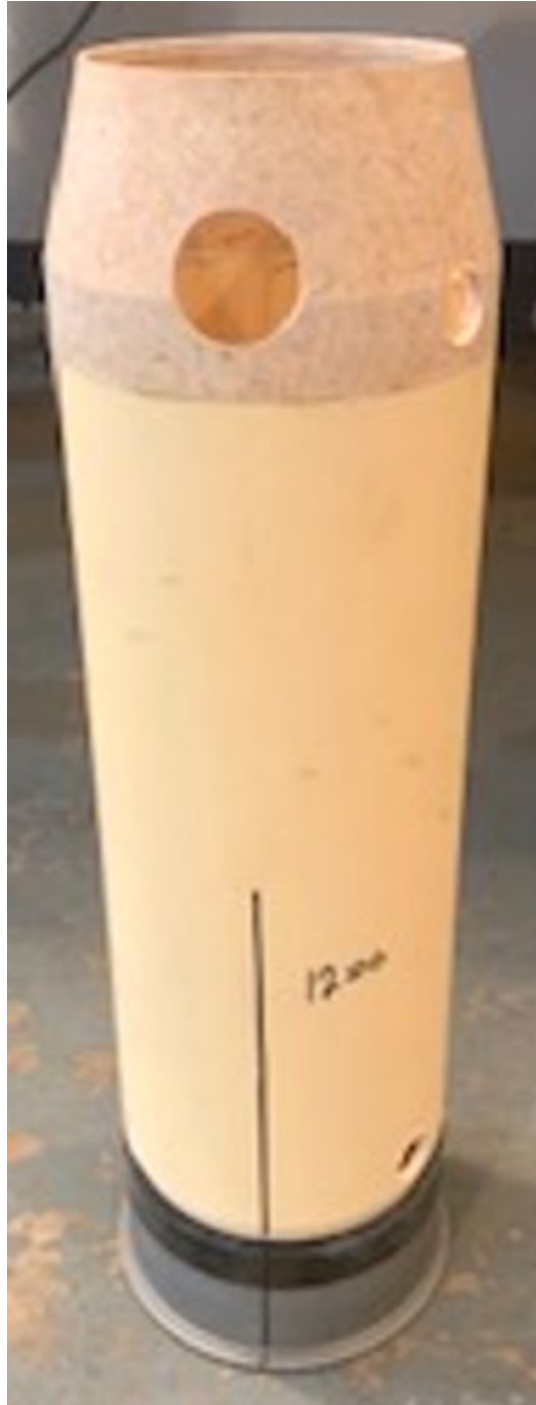
Fig. 4 12 o'clock sabot split markings on combustible case and stub base
