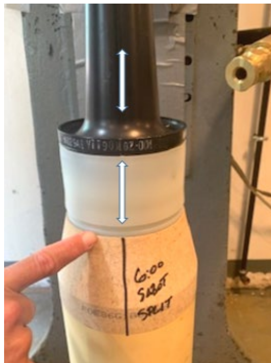
Fig. 8 Horizontal alignment of the obturator with the split of two sabot petals aligned with the 6 o'clock split line on the case adapter
