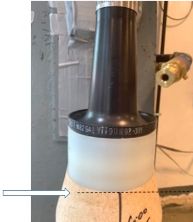
Fig. 10 Shown here is the proper result of an even assembly of the obturator and the case adapter, with no damage to the case adapter
