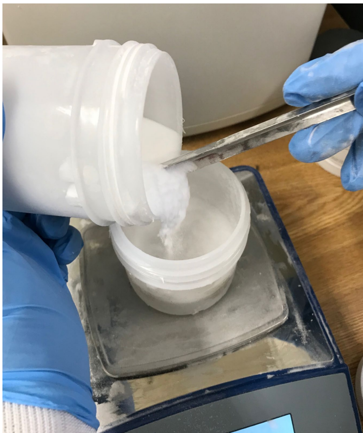
Figure 4. K1 glass microspheres were added to the 10:1 ratio of elastomer base and curing agent; approximately 150 mL of these microspheres were used in each cup
