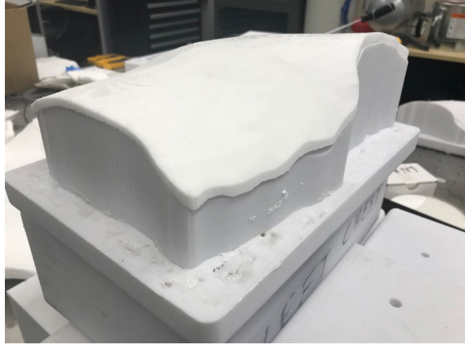
Figure 8. After curing, the top portion of the mold was removed, and the completed panel was extracted
