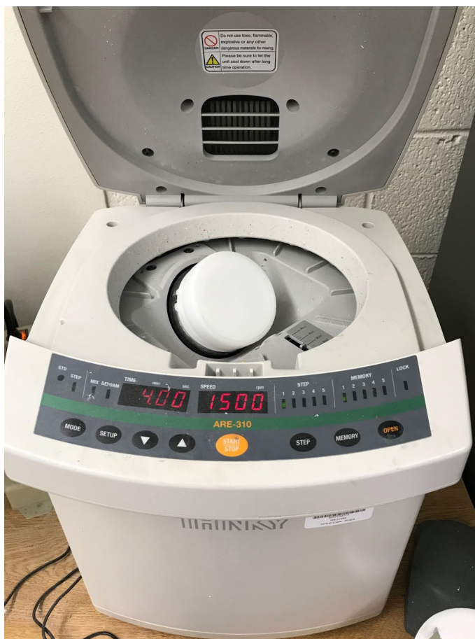
Figure 5. Composite mixtures were placed in a THINKY planetary rotary mixer for 4 min at 1500 rpm to allow for thorough mixing
