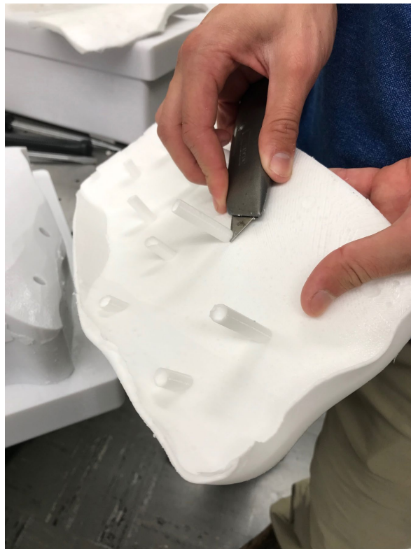
Figure 9. Excess material from the edges and mold shafts were trimmed from the extracted panel
