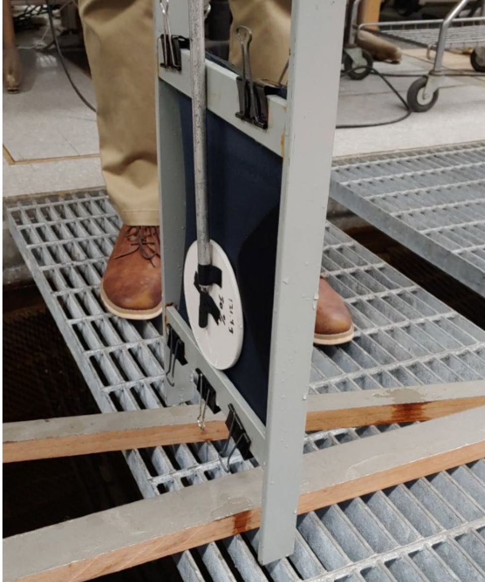
Figure 17. Hydrophone and composite puck arrangement behind neoprene material (held out of tank for visualization)
