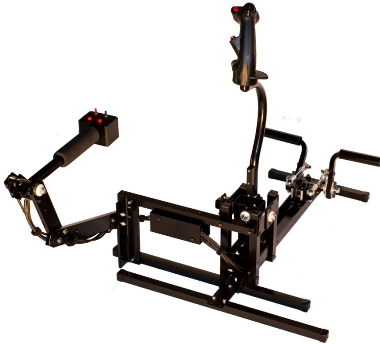
Figure 10. Pro Flight Training PUMA Helicopter Control Device. Source: Pro Flight Trainer (n.d).
