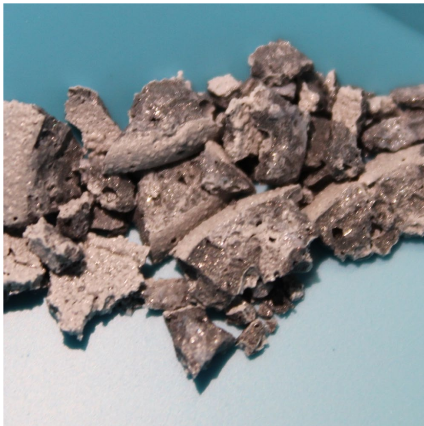
Figure 69. \text{ZrB}_2 held at 1300 °C for 1 hour. A Glassy film and an oxidation layer are observed on the sample.
