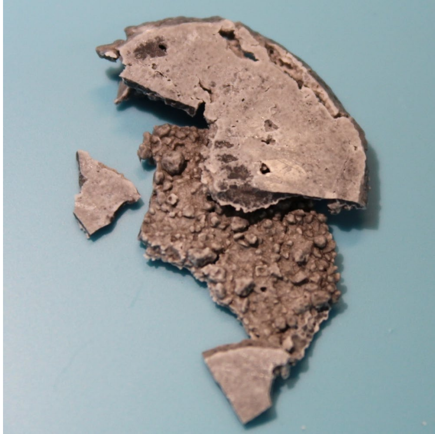
Figure 35. HfB 2 held at 1300 °C for ten hours.
