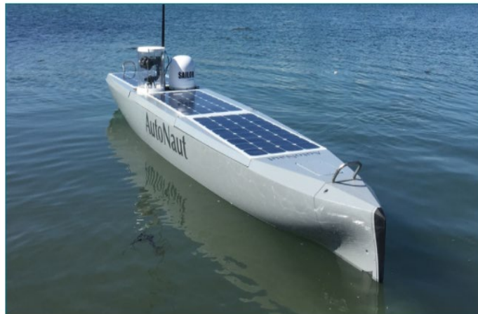
Figure 3. Auto Naut 3D printed vessel, built by laser sintering method. Source: [10].
