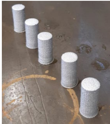
Figure 28. Solid cylindrical test specimen (solid infill)
