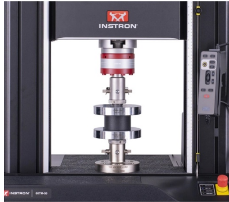
Figure 12. Instron compressive testing machine. Source: [22].
