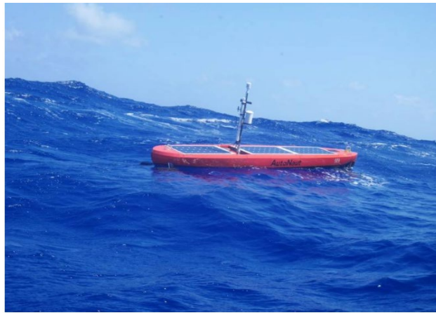
Figure 2. Auto Naut 3D printed vessel could capsize and self-right. Source: [9].
