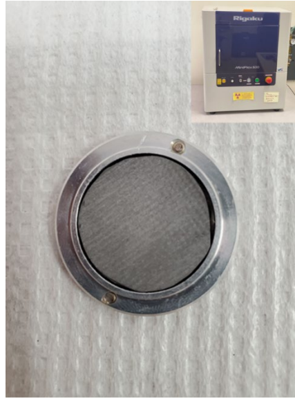
Figure 57. PLA specimen mounted in 24mm open tray and Rigaku Miniflex 600 XRD (inset)
