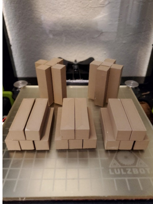
Figure 13. Bronze PLA printed compression test specimens. Foreground samples are printed in the XYZ direction. Samples in the back of the image are printed in the ZXY direction.
