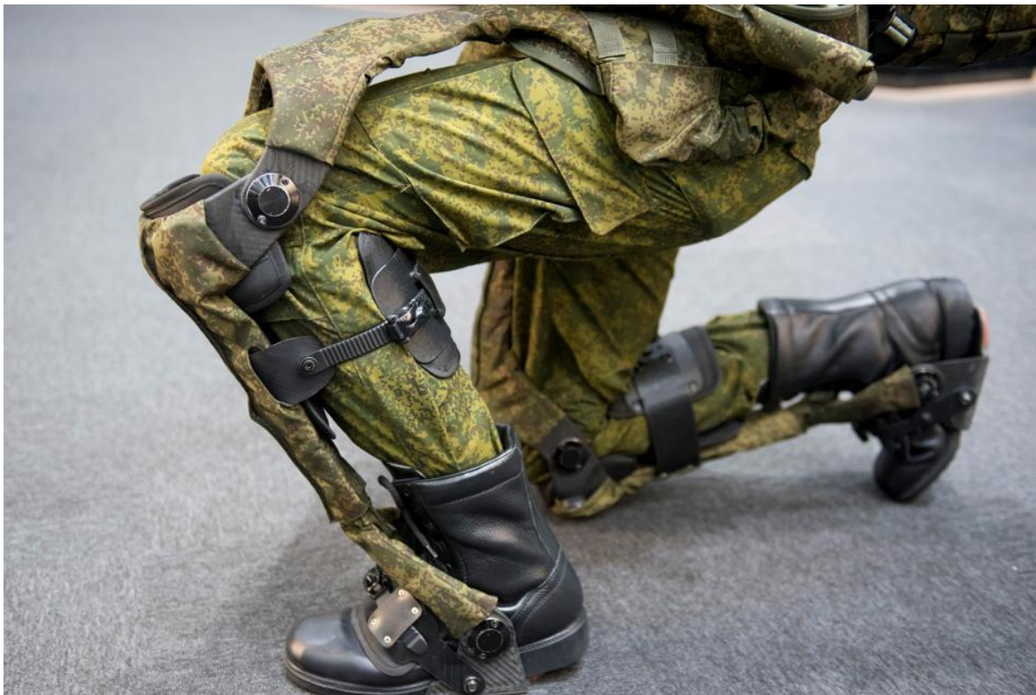
Figure 13. Example of ROSTEC's Ratnik Exoskeleton (passive)
