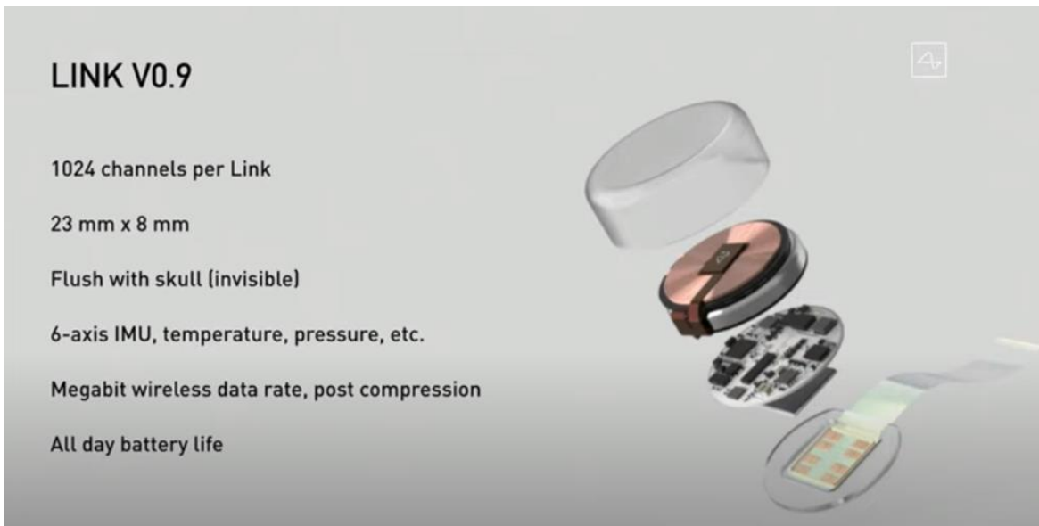
Figure 10. An overview of the Neuralink device, from the August 2020 live update
