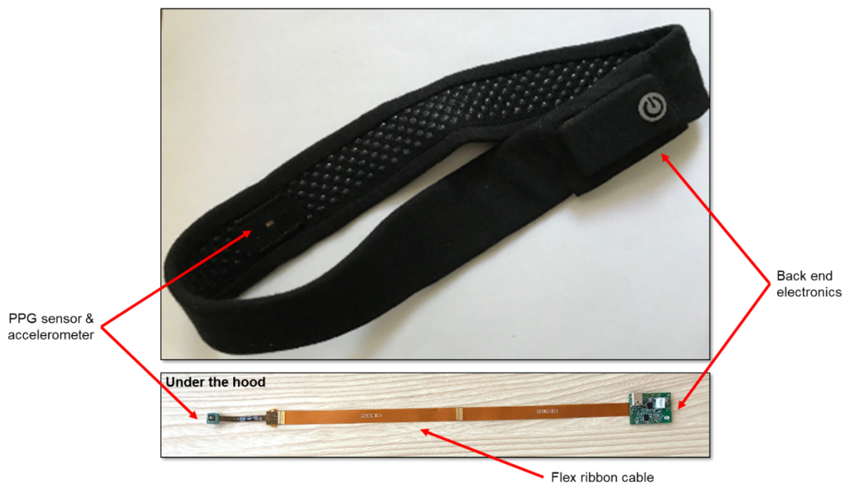
Figure 1. Textile integrated oximeter headband sensing device (top). Internal electronics (bottom).
