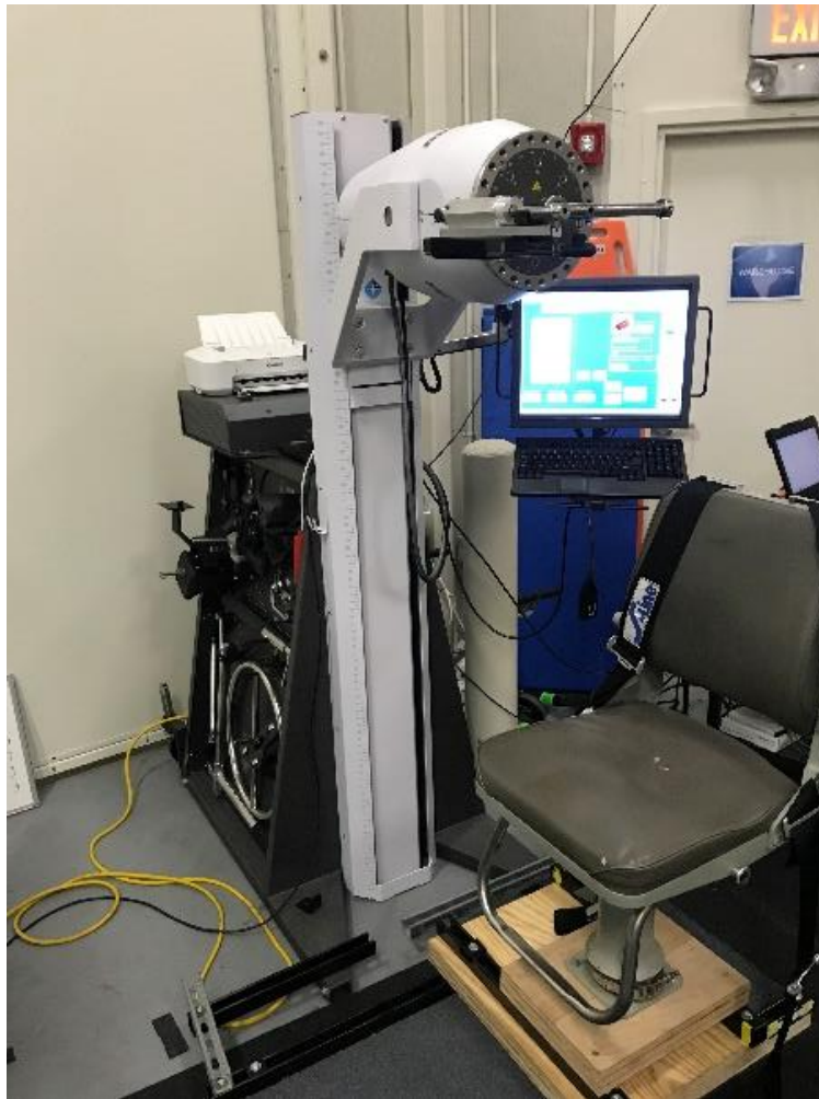
Figure 4. Dynamometer. The BTE PrimusRS with affixed chair used in conjunction with the custom-built MATLAB graphical user interface (GUI) to conduct and collect the dynamometer assessments (isometric strength, muscular control, and endurance).
