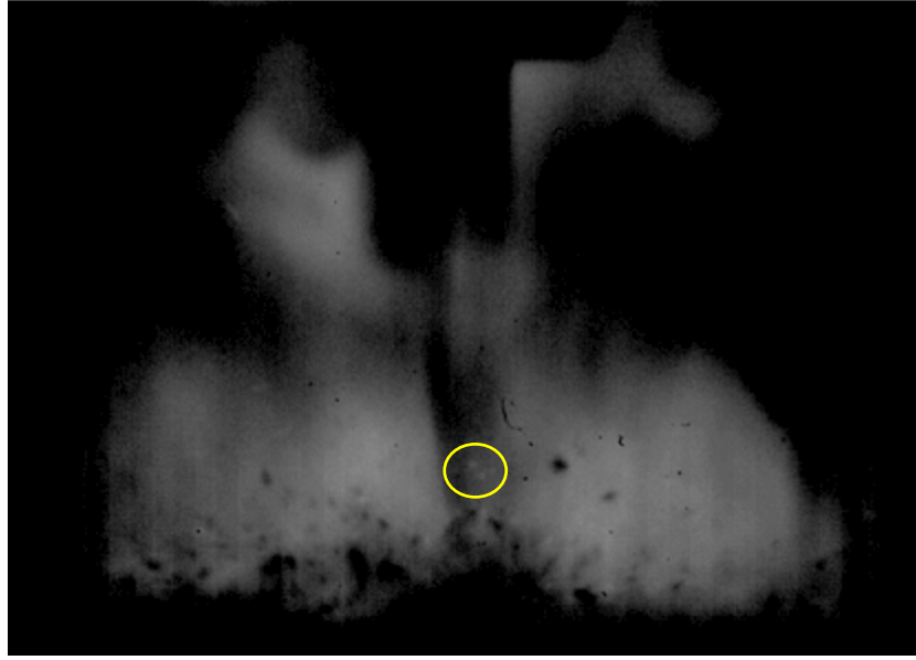
Fig. 11 Snapshot from the high-speed video of GO-coated nano-Al particles being ejected into the air 30 \mu s after being subjected to a 10.5-J discharge; the ejected particles appear black against the residual discharge emission since they are not burning, while a few smaller particles inside the yellow circle may be burning (picture has been cropped and the brightness/contrast adjusted)
