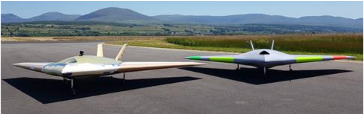
(d) MAGMA Conventional (Left) and MAGMA Fluidic (Right).
