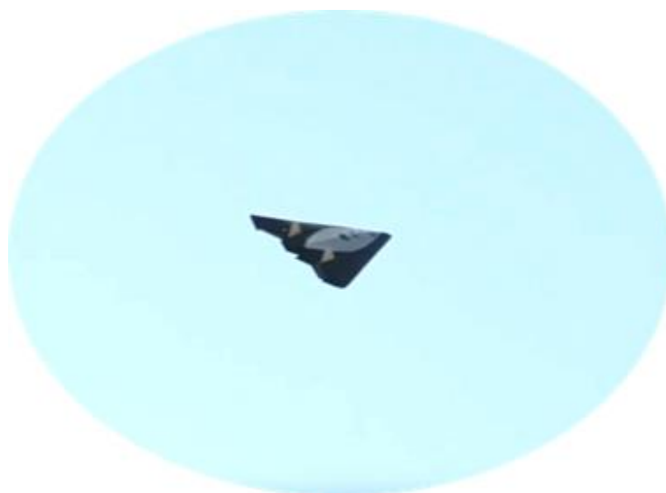
Figure 11-20: ICE 1/7th Scale Foam Test Aircraft in Flight.
