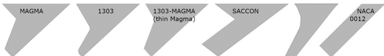
Figure 5-2: Four BWB Models (Left) and Two Swept-Back Wings (Right) Tested Using a Small Number of Sweeping Jet Actuators for the Purpose of Suppressing Spanwise Flow.
