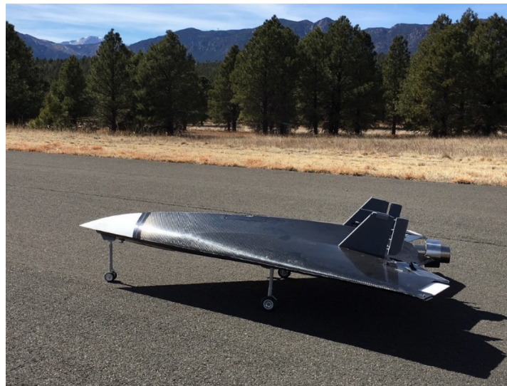
Figure 11-1: 1/7th Scale Carbon Fiber ICE Vehicle with AFC and Conventional Control Effectors.
