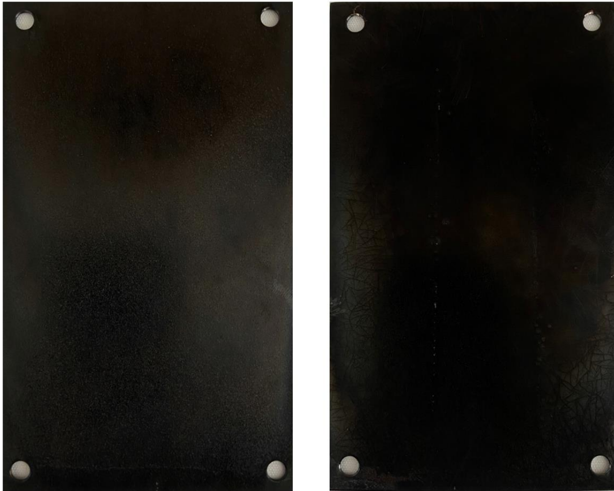
Figure 26. Samples blackened with alternative anodic oxidation. (Left) SN 101 aluminum panel (Right) SN 201 Invar 36 panel.
