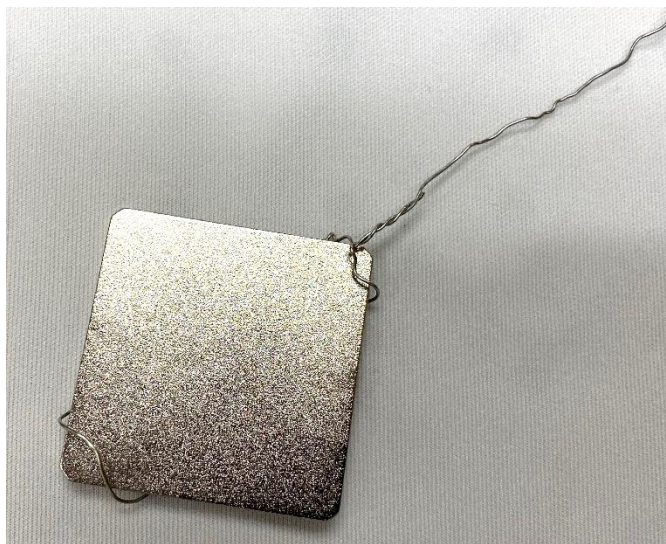
Figure 10. EN plated sample suspended with steel wire.
