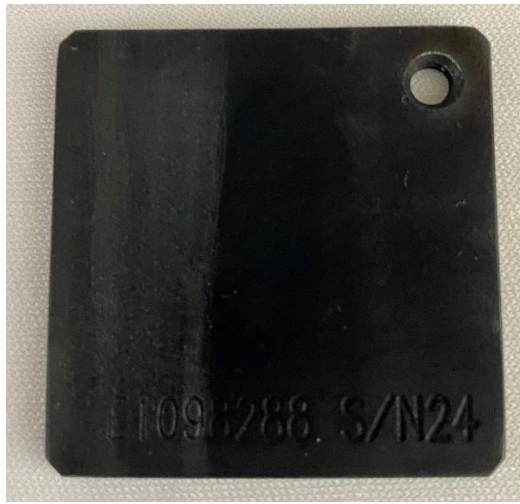
Figure 18. Black oxide deposit on surface of sample. Left side of image - deposit removed by wiping area with a clean, lint free cloth.
