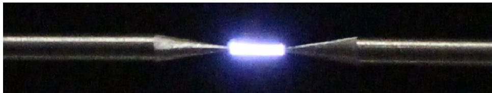
Figure 1: Single nanosecond pulse discharge within a pin-to-pin electrode separation of 2 mm
