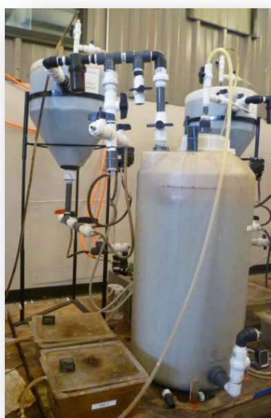
Two-stage pilot digester with bamboo biocarriers
