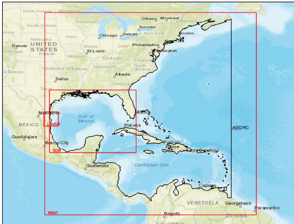
Figure 5. Map showing the three grid boundary extents for the regional wind and pressure files in (red) and the ADCIRC model domain shown in black.
