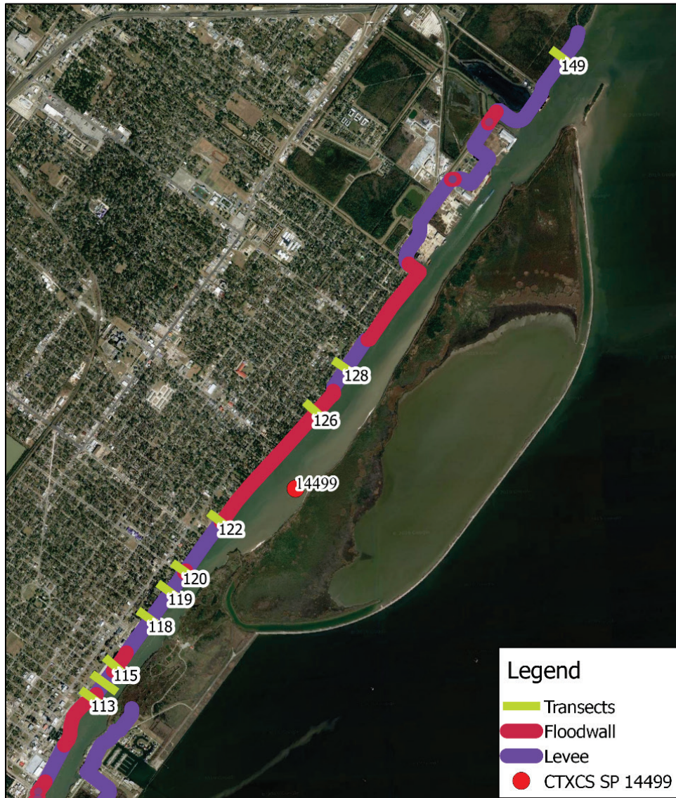
Figure 47. Locations of transects along the SNWW used for validation of runup and overtopping StormSim module.
