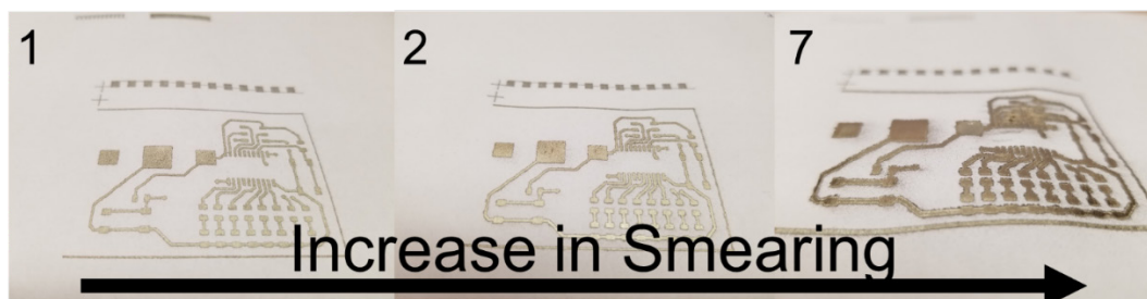
Figure 5. Printed surfaces as a function of number of passes of the same design. Substrate was cellulose for each. Number on each image indicates the number of passes.
