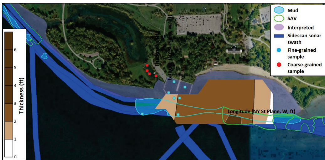
Figure 14. Example of data interpolation. Fine-grained regions and SAV-dominated regions (light blue and green polygons, respectively) were digitized directly on the sidescan sonar swath (dark blue polygon) and imported into Google Earth. Sediment samples are plotted as blue and red circles for dominantly fine- or coarse-grained, respectively. Regions that were not mapped due to limitations in vessel draft but that are interpreted to be fine-grained are plotted as purple polygons. Please note that these color conventions are the same for Figures 16–25, below.
