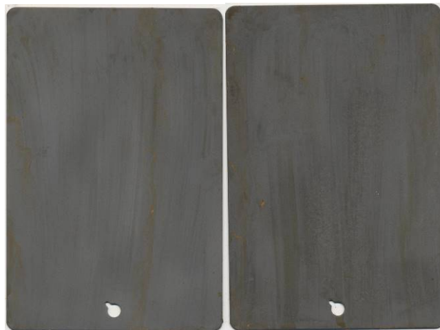
Fig. 8 Type Z, Class 2 coupon sealed with SurTec 580 (L) and SurTec 590 (R)
