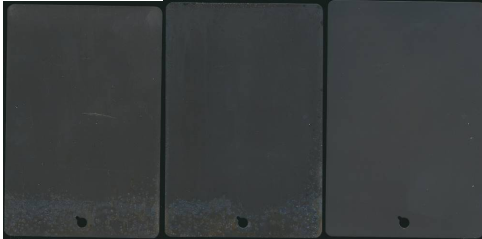
Fig. 6 (L to R) Type M, Class 3 coupon sealed with Bonderite M-CR T5900, SurTec 555, and SurTec 590
