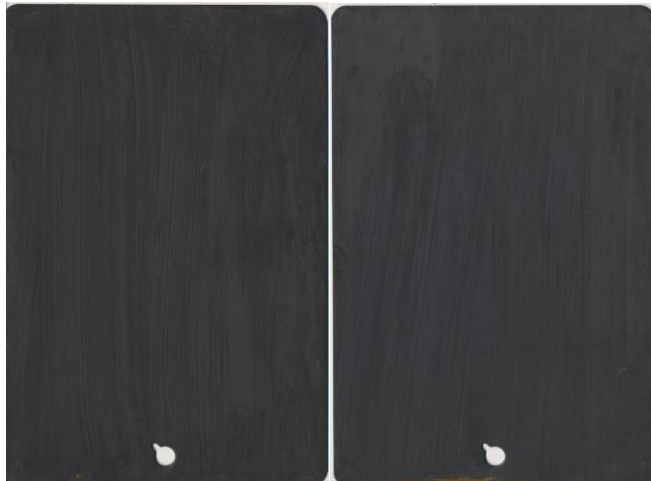
Fig. 7 Type M, Class 2 coupon sealed with SurTec 580 (L) and SurTec 590 (R)
