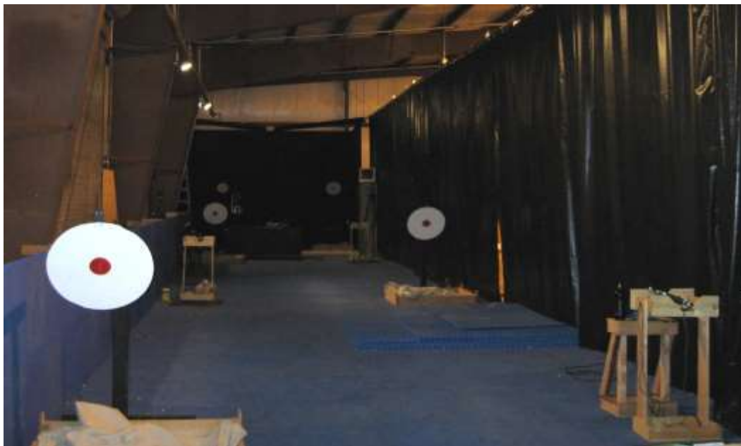
Figure 4 Experimental approach arena with shooting stations, targets, and marksman's station (threat source) at the far end
