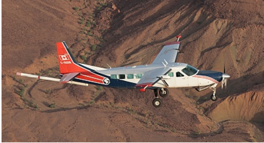
Figure 7: Tail-mounted stinger on a geo-survey aircraft [20].
