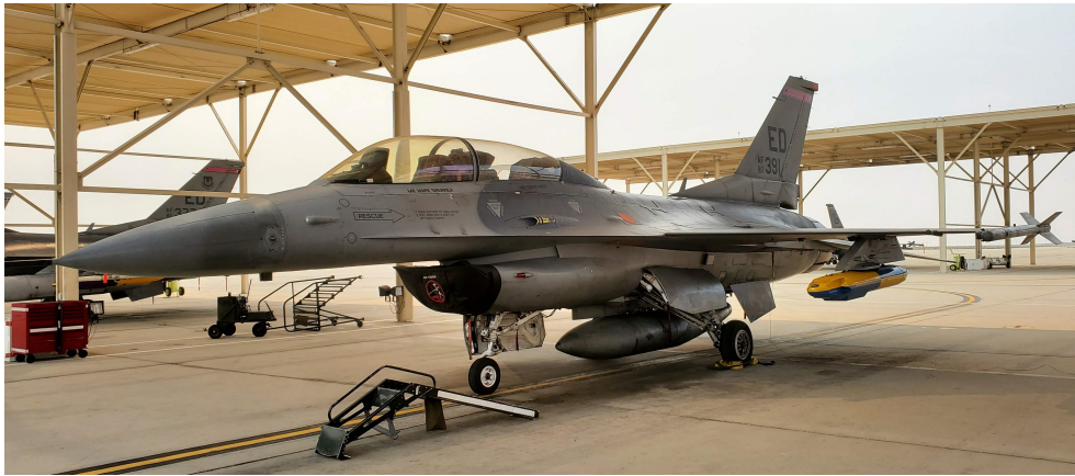
Figure 24: USAF F-16 aircraft carrying TPS’s RASCAL pod. The F-16 with RASCAL pod was used to collect the F-16 magnetic field data set.
