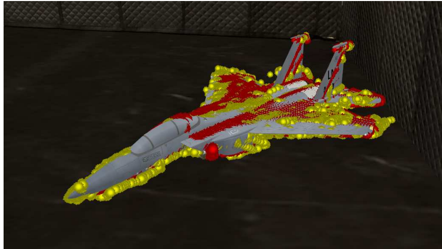
Figure 26: Shelled Reference Model (Red) Matched to Sensed Points (Yellow) MCS Truth Data is the Textured Aircraft Model
