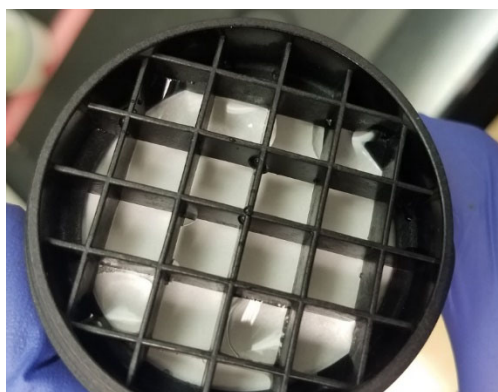
Figure 4. Wet membrane experimental setup.
