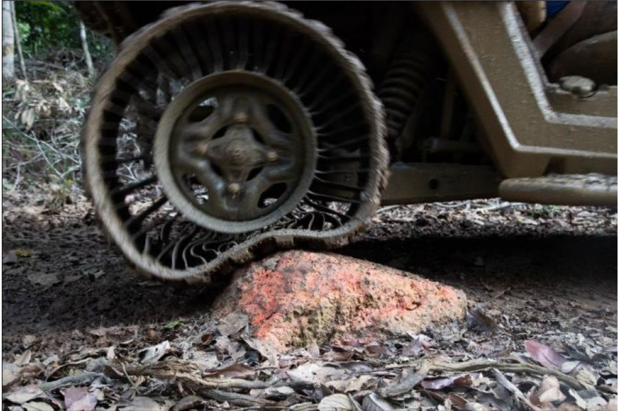
Caption: Airless Developmental Test in Suriname—obstacle crawling deflection.
