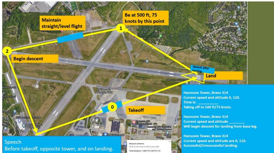
Figure 4. Traffic pattern protocol executed by participants for nominally 90 continuous minutes of flight.
