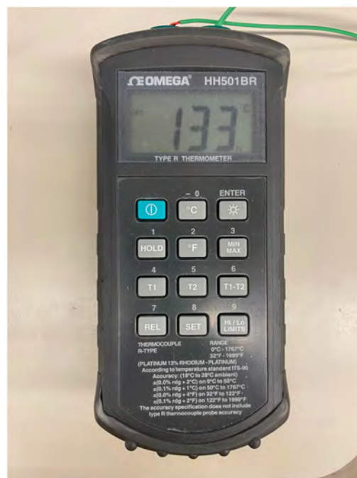
Figure 29. Omega HH501BR Thermometer used in AMTECO furnace temperature calibration
