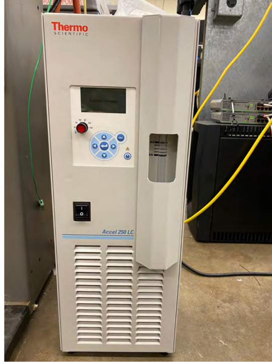
Figure 12. Thermo Scientific Accel 250 LC, Chiller used to regulate grip temperature
