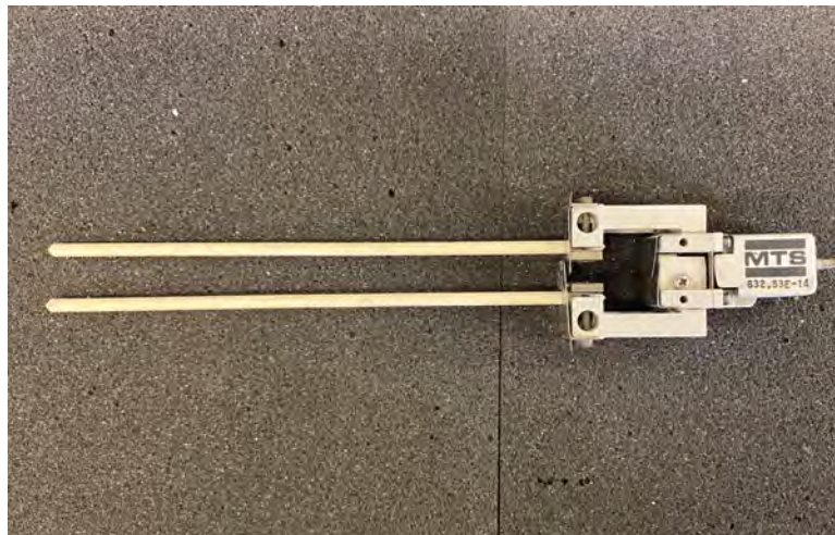
Figure 17. Low-contact force high-temperature MTS extensometer used to measure strain
