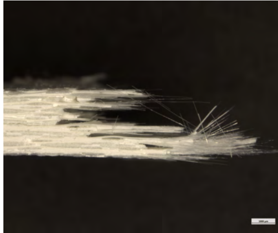
Figure 90. Optical micrograph of a N720/A specimen fracture surface tested in tension-tension fatigue at 1200°C in steam. \sigma_{\max} = 150 MPa, N_f = 700
