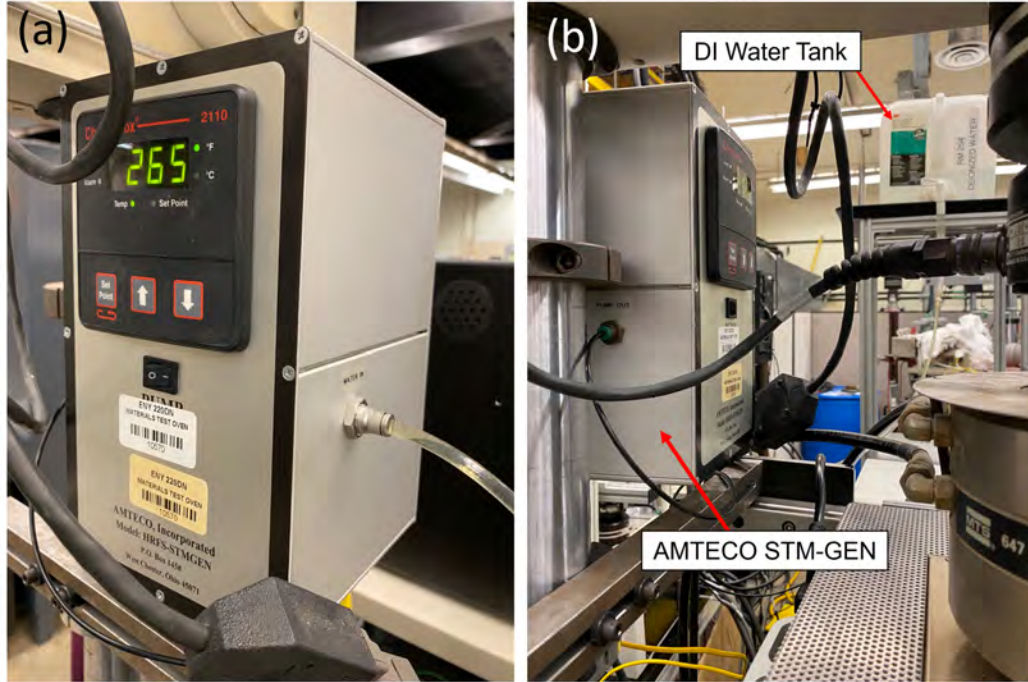
Figure 18. (a) AMTECO HRFS-STMGEN, Steam Generator/Pump, with Chromalox 2110 Temperature Controller, (b) Steam Generator with DI Water Holding Tank and feed tube
