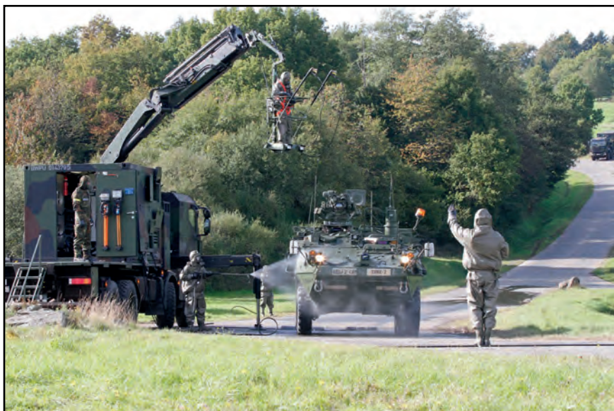
Countering CBRN Field Training Exercise GOLDEN Mask in Baumholder, Germany. Nuclear Biological Chemical Reconnaissance Vehicle (NBCRV) Stryker assigned to the Regimental Engineering Squadron, 2nd Cavalry Regiment, is decontaminated by a German TEP-90 trailer-mounted mobile decontamination system. (Photo courtesy of the Bundeswehr CBRN Defence Command)
