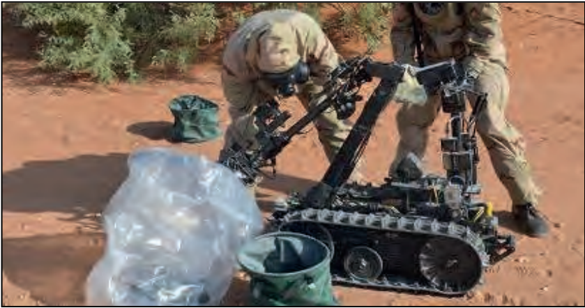
US Chemical operation specialists with the 83 rd Chemical Battalion, Fort Stewart, Georgia, ensure that the Talon robot is decontaminated after completing a chemical analysis. (Photo by Justin Geiger, courtesy of the US Army 7 th Mobile Public Affairs Detachment)
