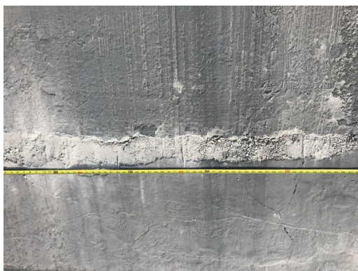
(e) Spalling in Quadrant #3 at 784 passes
