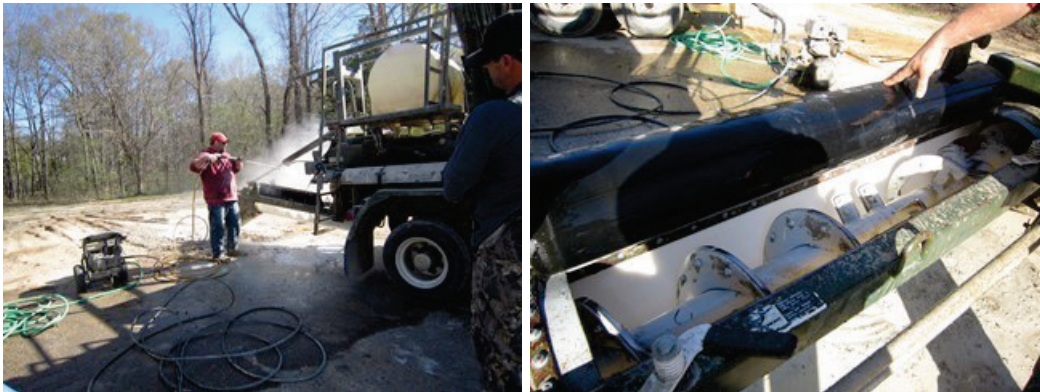
Figure 33. Washout of volumetric mixer using a pressure washer (left) and the resulting clean auger (right).
