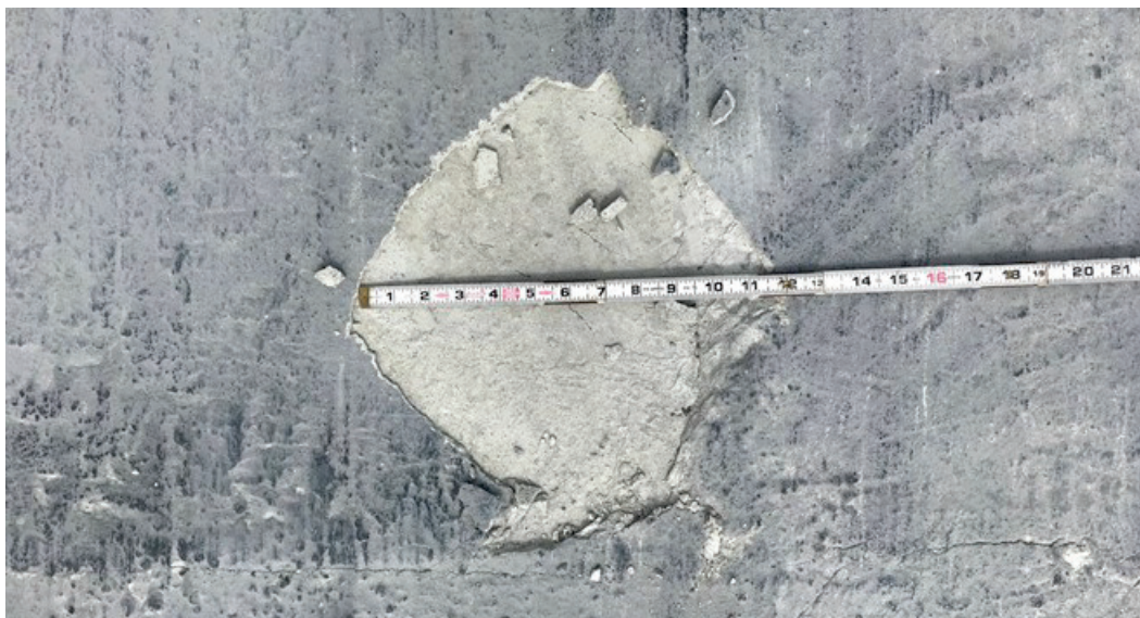
Figure 52. Overview of Repair 6 at 2,112 passes.
