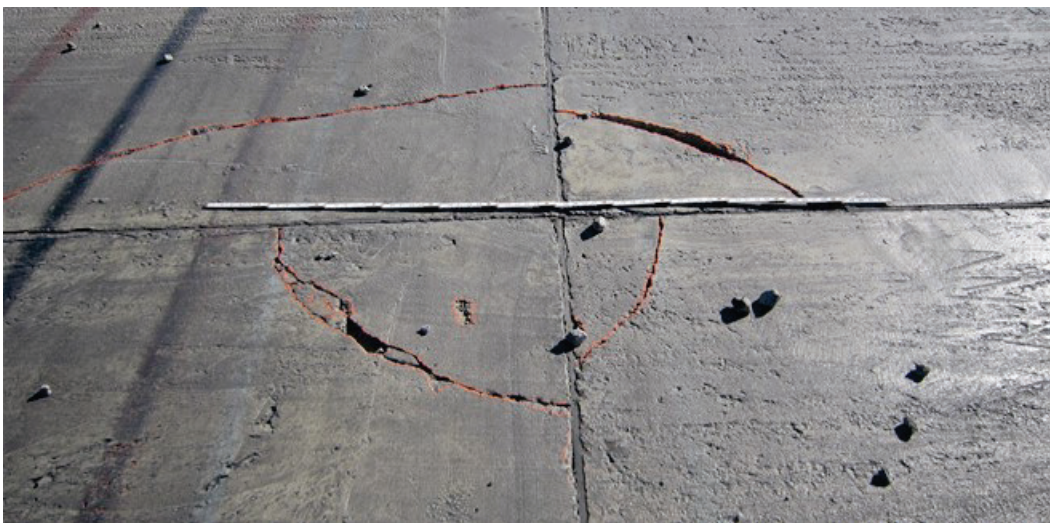
Figure 36. Large 2-in. FOD after 1,680 passes, in the center of Repair 1.
