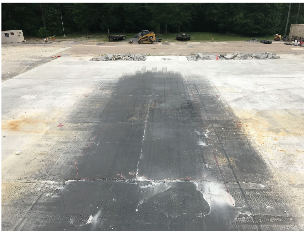
Figure 52. Overview of Repair 6 at 2,112 passes.
