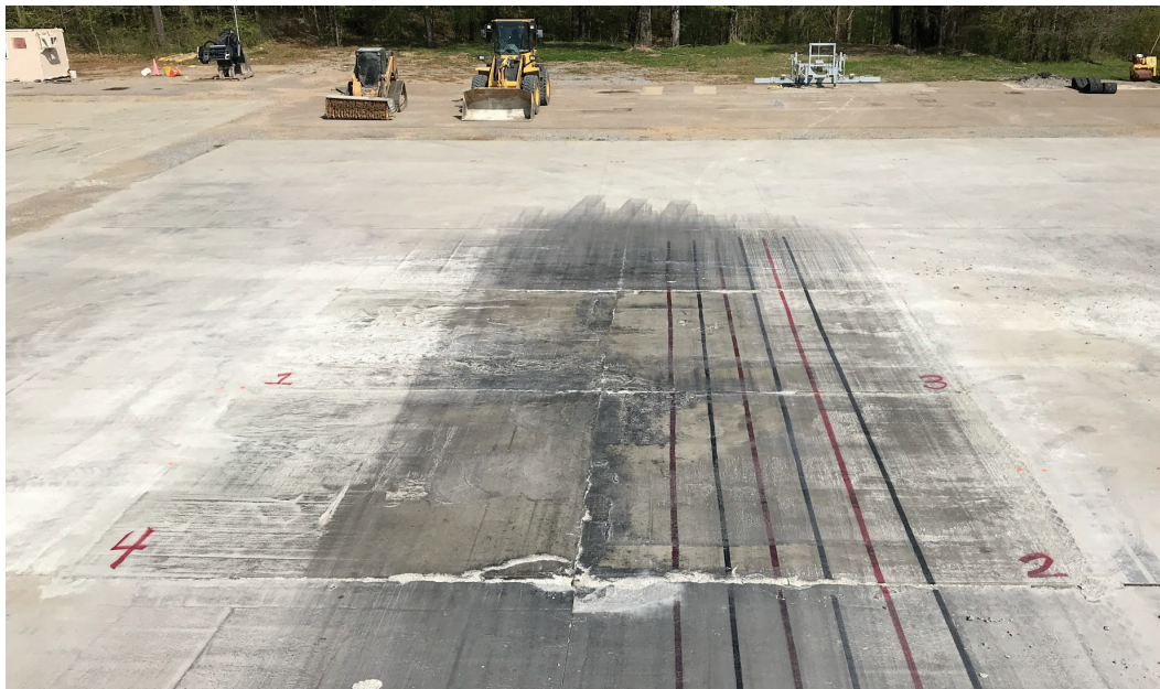
Figure 49. Overview of Repair 5 at 274 passes.
