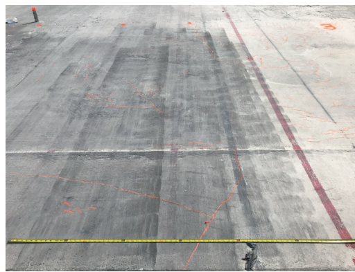
(b) Cracking in the paste at 112 passes
