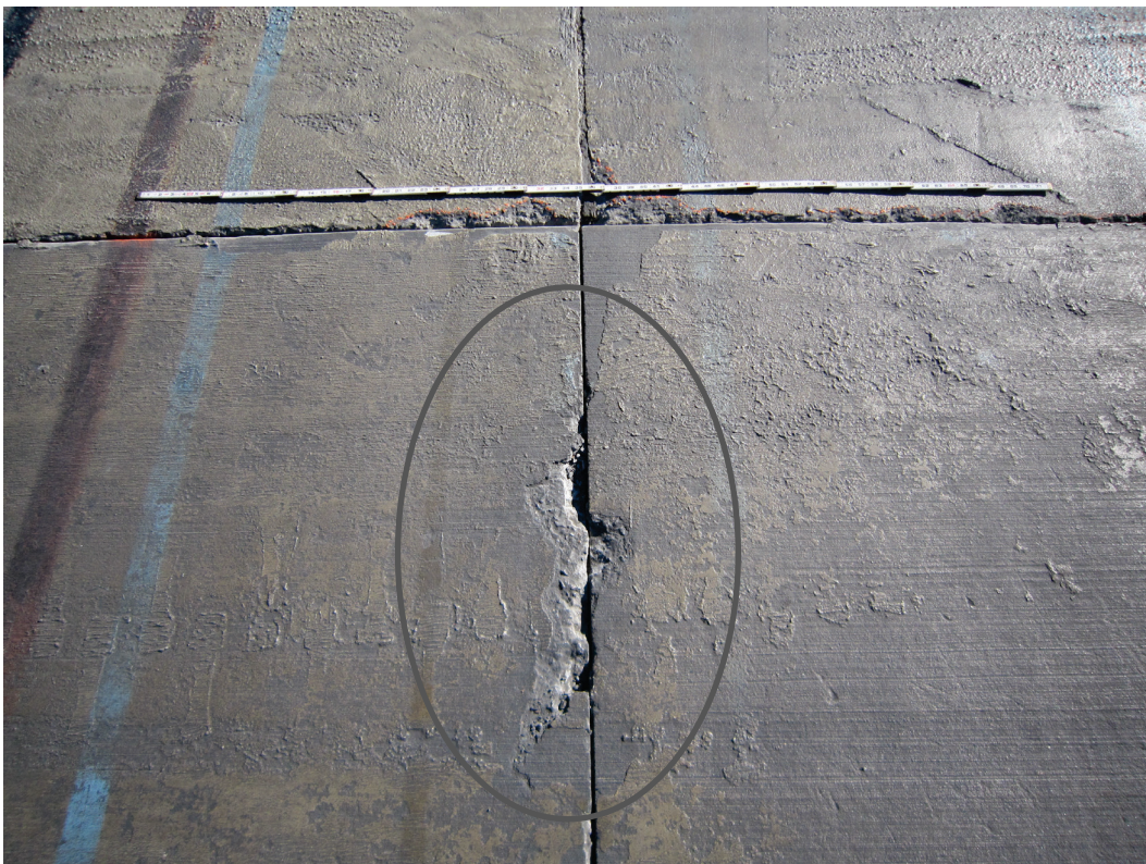
Figure 38. Parent slabs adjacent to the repair started to spall after 1,680 passes.
