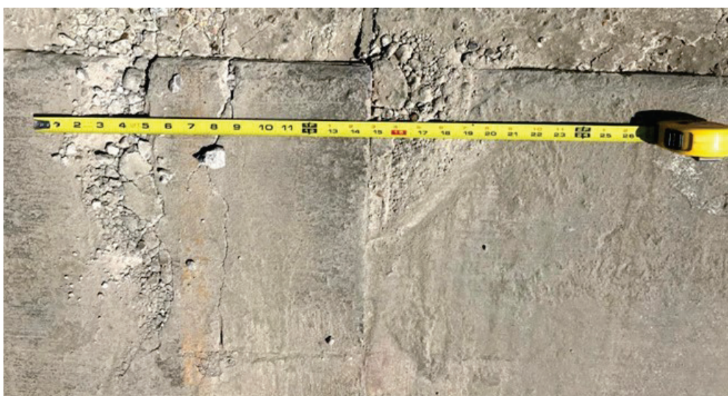
Figure 41. Spalling on parent slab in the trafficking area at 224 passes.
