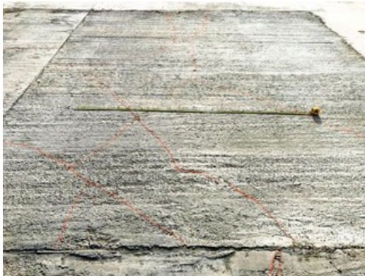
(b) Low severity shattered slab at 112 passes
