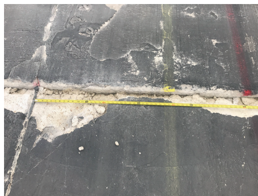
(f) Spalling in Quadrant #3 at 896 passes
