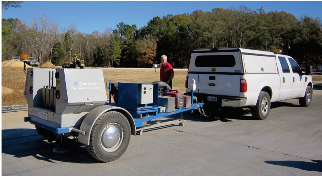
Figure 6. HWD testing on a large crater repair.
