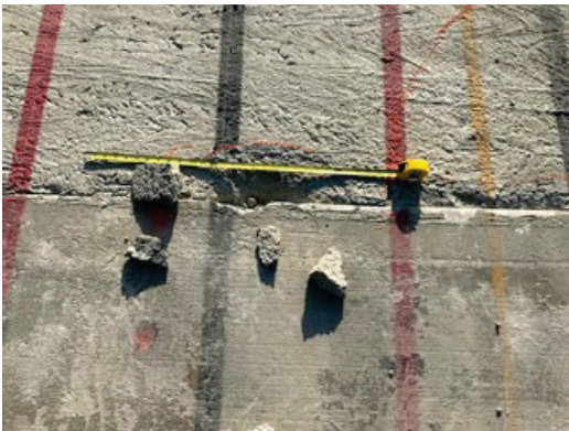
(c) FOD and spall on the western edge at 112 passes
