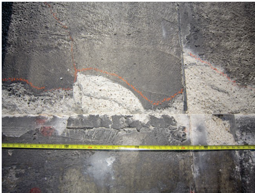
Figure 47. Western edge of Repair 4 after 336 passes.
