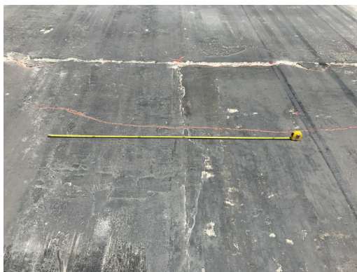
(e) Crack from Quadrant #1 to #3 at 768 passes
