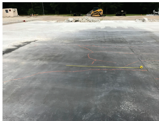
(f) Low-severity shattered slab in Quadrant #1 at 1,664 passes
