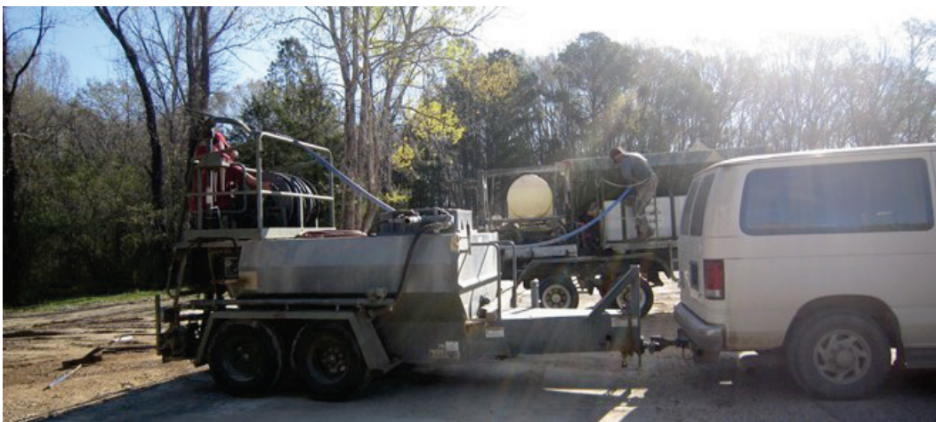
Figure 32. Refilling volumetric mixer water tanks (background).
