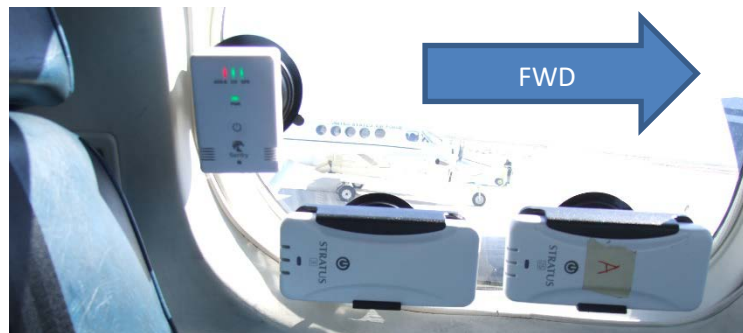
Figure 8: C-12 AHRS Capable SUT Installation
