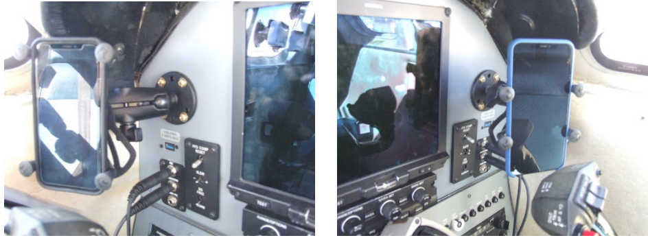
Figure 9: C-12 Cellphone SUT Installation
