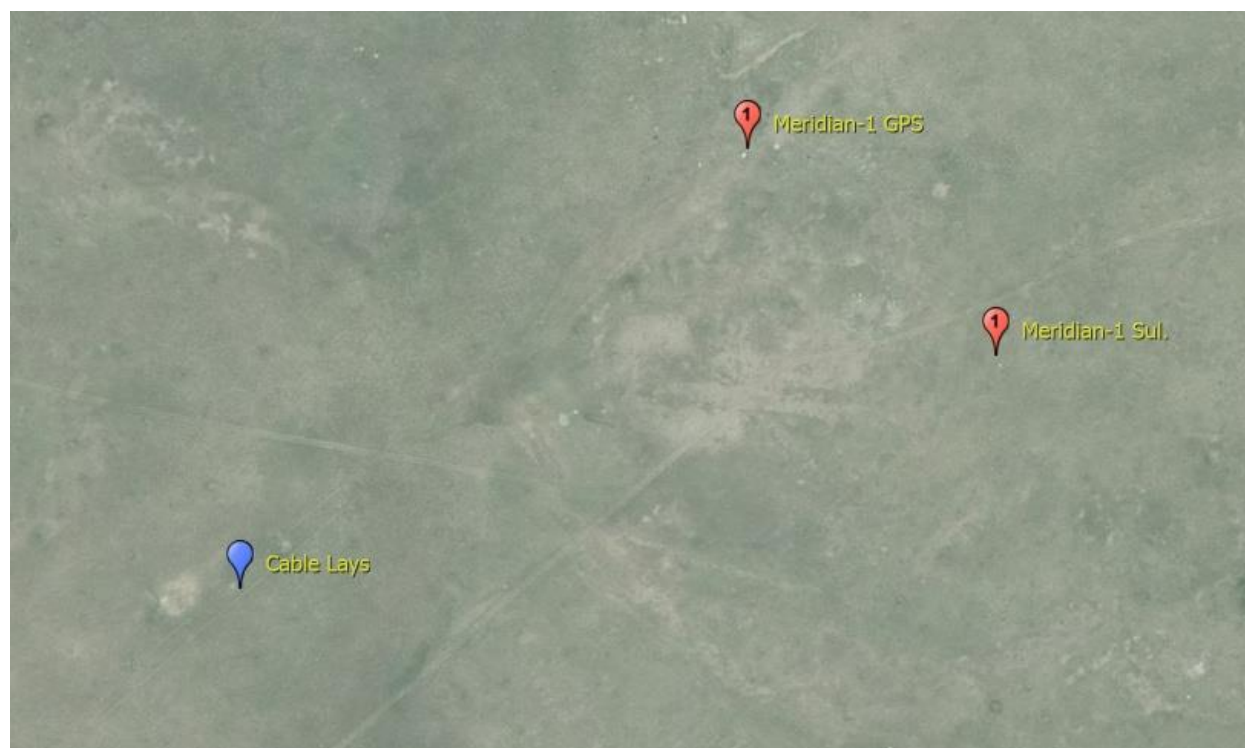
Figure 71. Overview of the Meridian-1 site from Bing Maps. The Sultanov et al. (1999) location is shown slightly to the southeast of the GPS coordinates obtained by field inspection of the site. The small white dot below the GPS location marker is the borehole. The two adjacent white dots are concrete pads probably used for erection of a support. Extending southwest from the GPS location are two parallel lines which are probably cable trenches for signals to the experiment control site.
