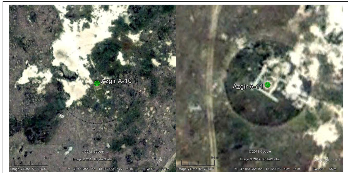
Figure 10. Google Earth images of the Azgir A-10 and A-11 sites showing the typical ring or presumed fence that we interpret as enclosing the borehole locations for the Azgir tests.
