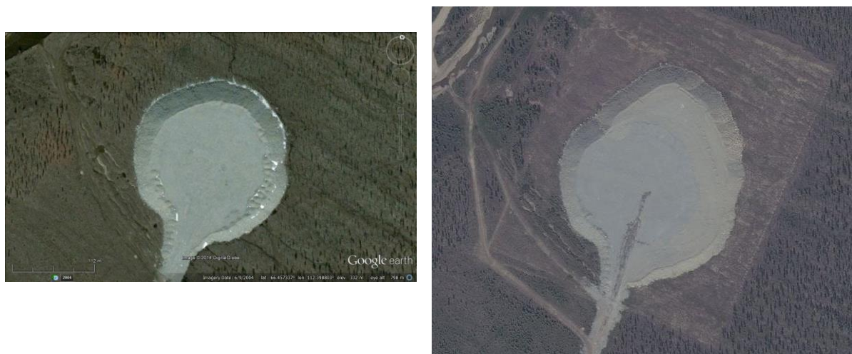
Figure 91. Satellite imagery showing the expansion of the shield covering the Crystal PNE site. The older image on the left is from Google Earth while the newer image, on the right, is from Bing Maps and shows that the shield is considerable expanded.
