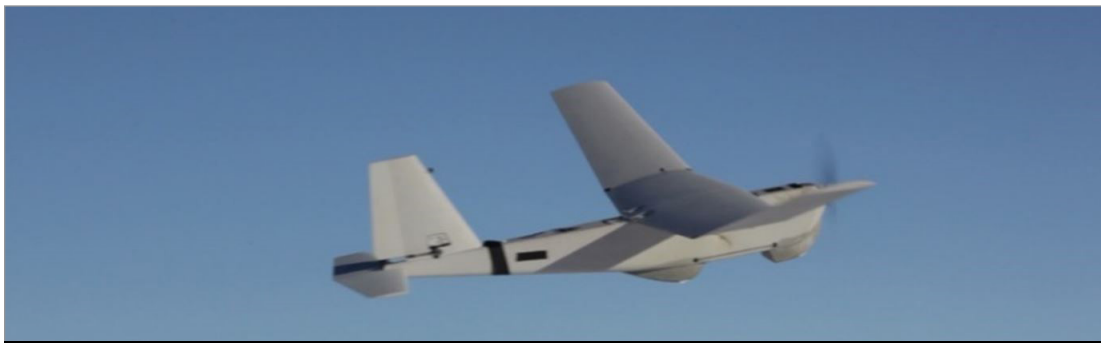
Figure 12. RQ-20A Digital Data Link Puma Block II Unmanned Aircraft Source: AeroVironment, Inc.
