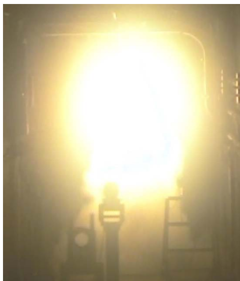
Figure 10. Testing of illumination candle at NSWC Crane photometric light testing tunnel.
