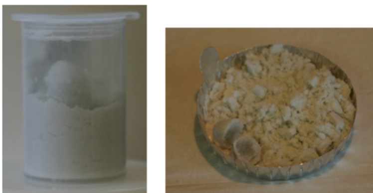
Figure 18. Images of early inert mixing attempts resulting in binder rich areas.
