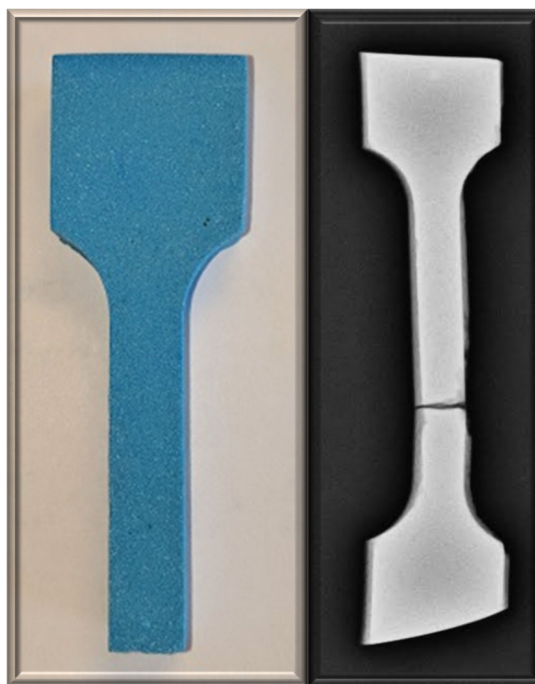
Figure 31. Typical cured PBXN-110 surrogate dog bone (left) and X-ray image of the same (right).
