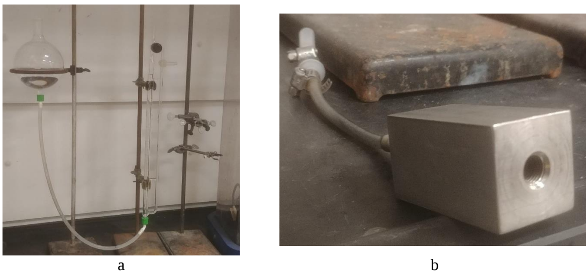
Figure 6.8. (a) Gas generation testing fixture used to test gas volume produced by delay formulations. (b) Closed combustion bomb used for ignition A-1A and delay material.
