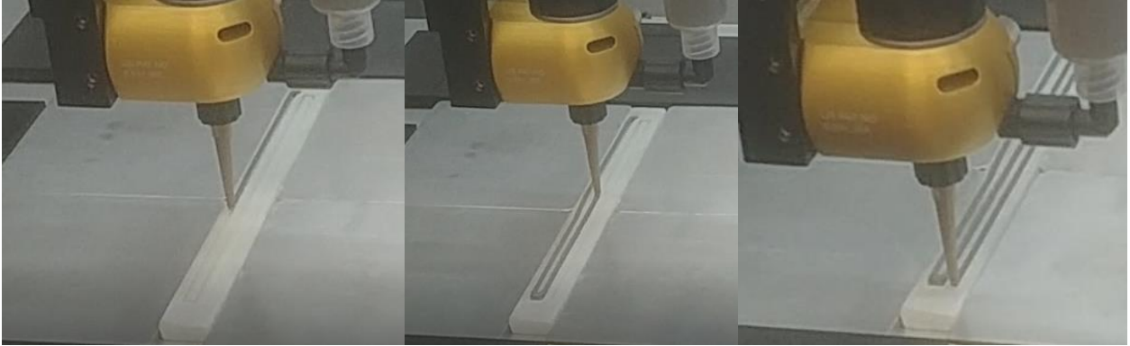
Figure 7.12. Depositing delay slurry onto substrate for new dispensing technology investigation.
