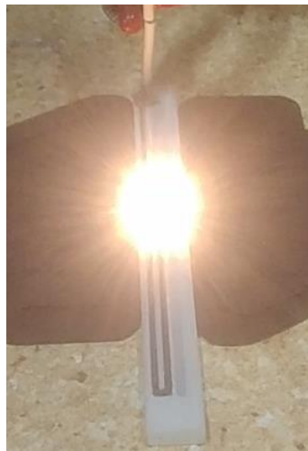
Figure 7.13. Image of combustion experiment of deposited delay slurry.
