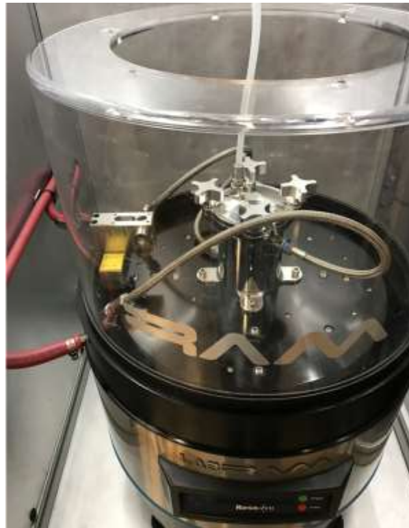
Photograph 7.2.5-1: Vessel with Cooling Jacket Secured to Mixer
