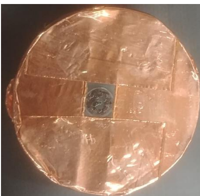
Figure 12.1. Stem of an M213/M228 fuze with combusted delay residue pressed into phenolic resin puck for SEM EDS mapping.
