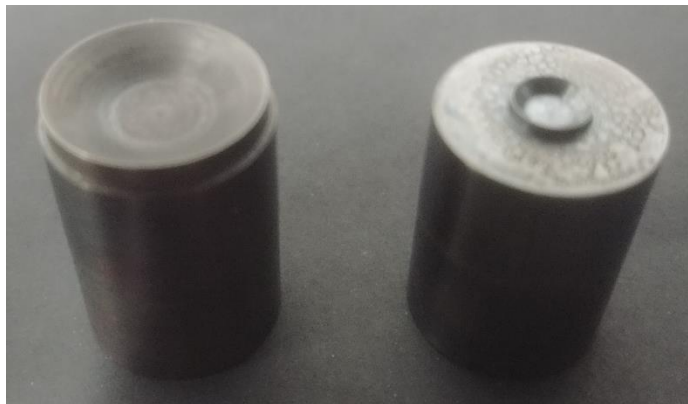
Figure 15.3. M213/M228 fuze primer holder assembly crimping die (left) and M42 primer crimping die (right).
