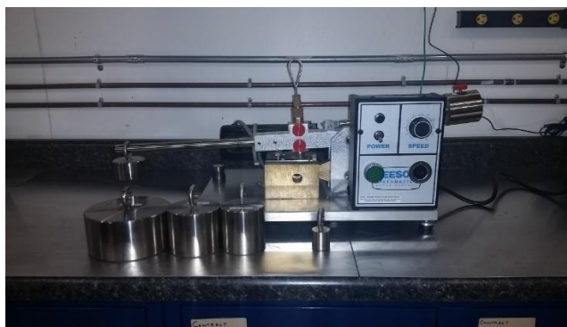
Figure 14.2. Photograph showing BAM friction sensitivity tester at Innovative Materials and Processes, LLC (Purchased from Chilworth Technology Ltd.).
