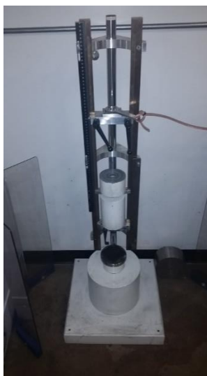
Figure 14.1. Photograph showing the BAM impact sensitivity tester at Innovative Materials and Processes, LLC (Purchased from Chilworth Technology Ltd.).
