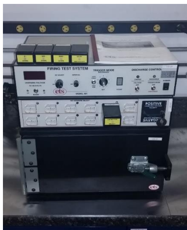
Figure 14.3. Photograph showing the electrostatic discharge tester with blast chamber at Innovative Materials and Processes, LLC (The manufacturer is Electro-Tech Systems Inc. Model 931).
