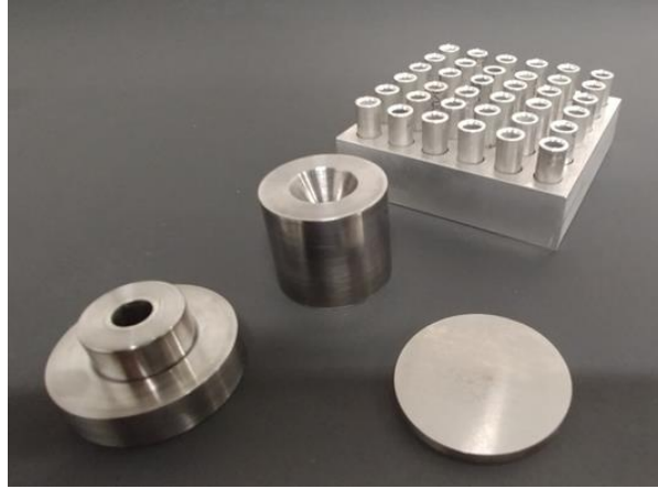
Figure 6.13. Photograph of mock delay column with the manufacturing and consolidation die.
