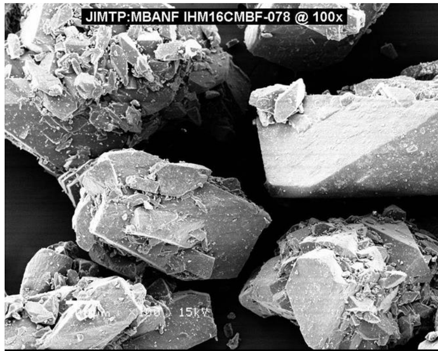
Figure 8.1. SEM Image of Recrystallized MBANF
