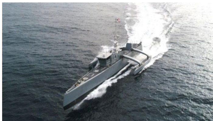
Autonomous Sea Hunter drone warship with CFRP hull
