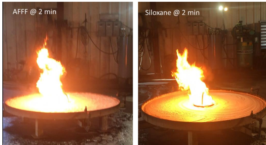
Figure 12. Burn-back testing images (A) AFFF and (B) MMI-Siloxane with additive after 2 minutes of the start of the testing. Siloxane formulation passed the “ad hoc” test with stability over 6 minutes.
