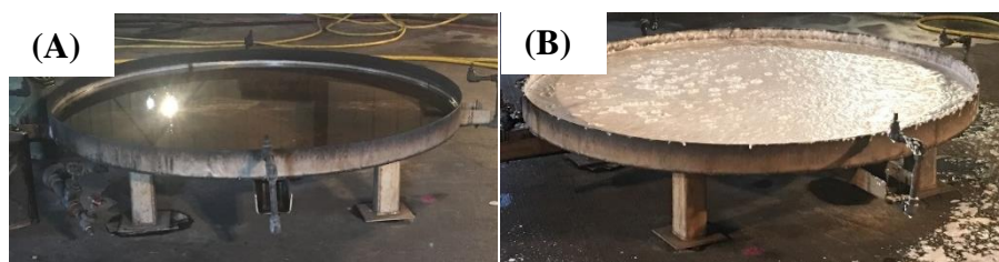
Figure 4. 6 ft diameter pool fire pan with (A) Fuel and (B) Foam on top of fuel after the extinction of fire
