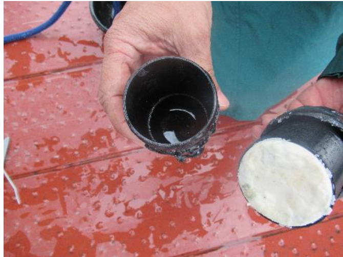
Figure 18. Water Inside EGP Device after Submersion
