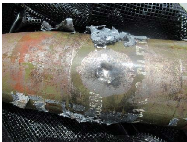
Figure 17. Poor Case Penetration
