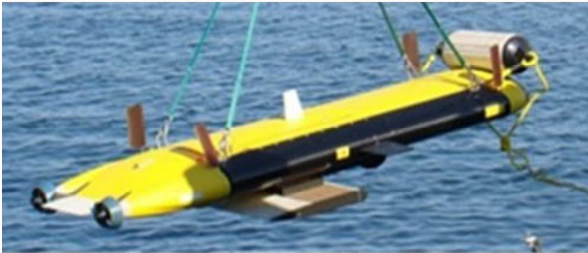
Figure 46. Razor AUV with eBOSS. Four 16-channel wing tiles are mounted below the across track wing. A Corprene signal conditioning plate / baffle (not shown) suppresses surface reflections.
