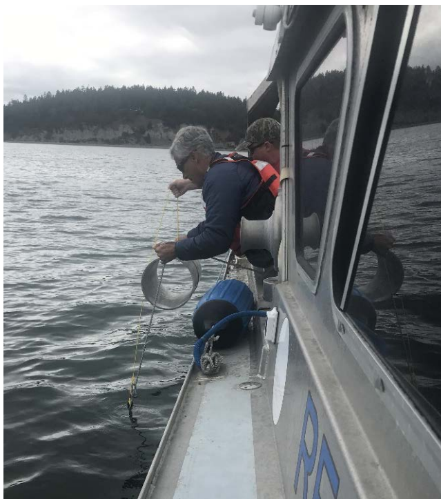
Figure 4. Deployment of the hollow aluminum cylinder by attaching it to the upline and sliding it down to the bottom.
