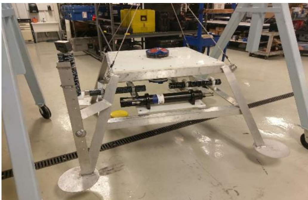
Figure 6: Instrument frame developed for MR-2730. Shown here with Teledyne RDI Sentinel ADCP, Nortek Aquadopp HR PC-ADCP, AML Plus-X CTD, and Imagenex 881 Tilt-Head rotary sonar.
