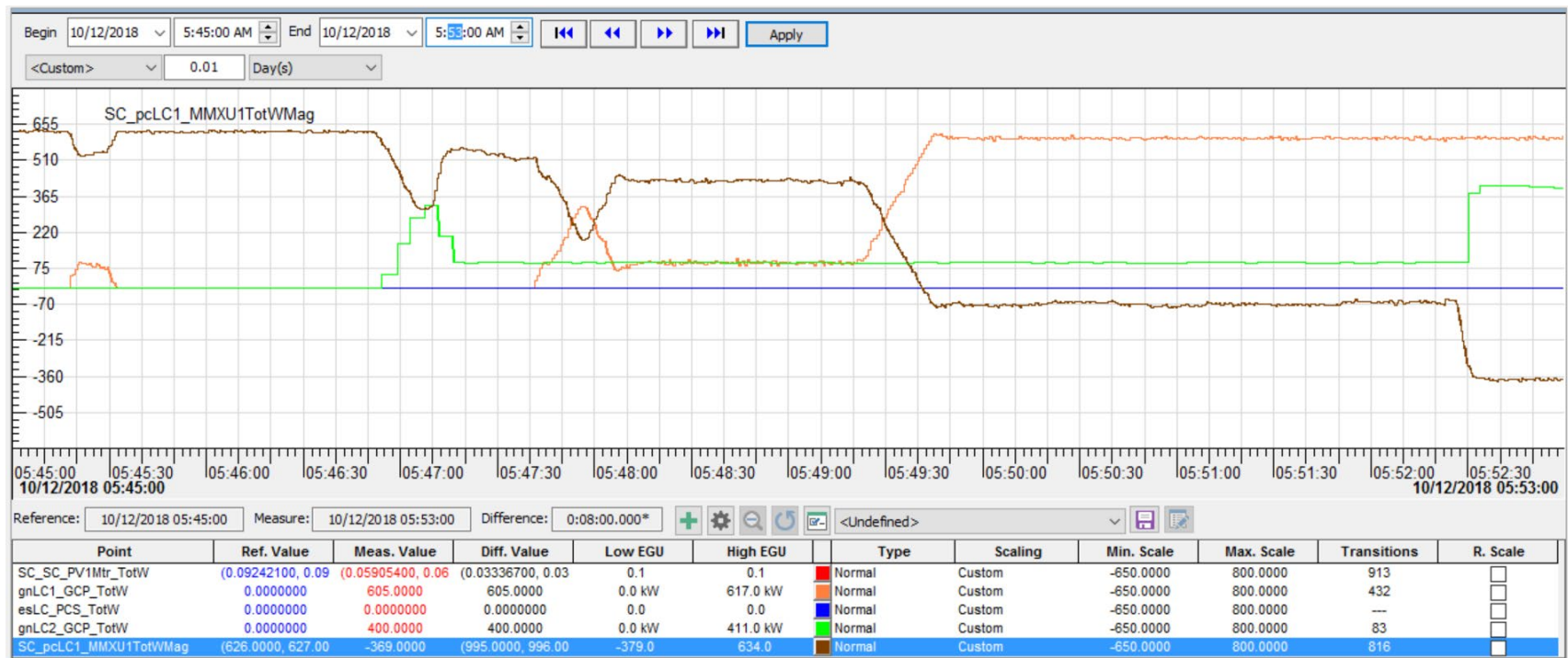
Figure 24. Real Power Output by Component for Grid Operation Initiation
