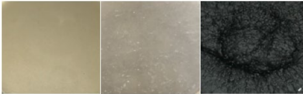
Figure 6. Digital Photograph of (a) Liquid PCM Mixture, (b) Gel PCM (c) Thermal Enhanced PCM with the Addition of Nanomaterials
